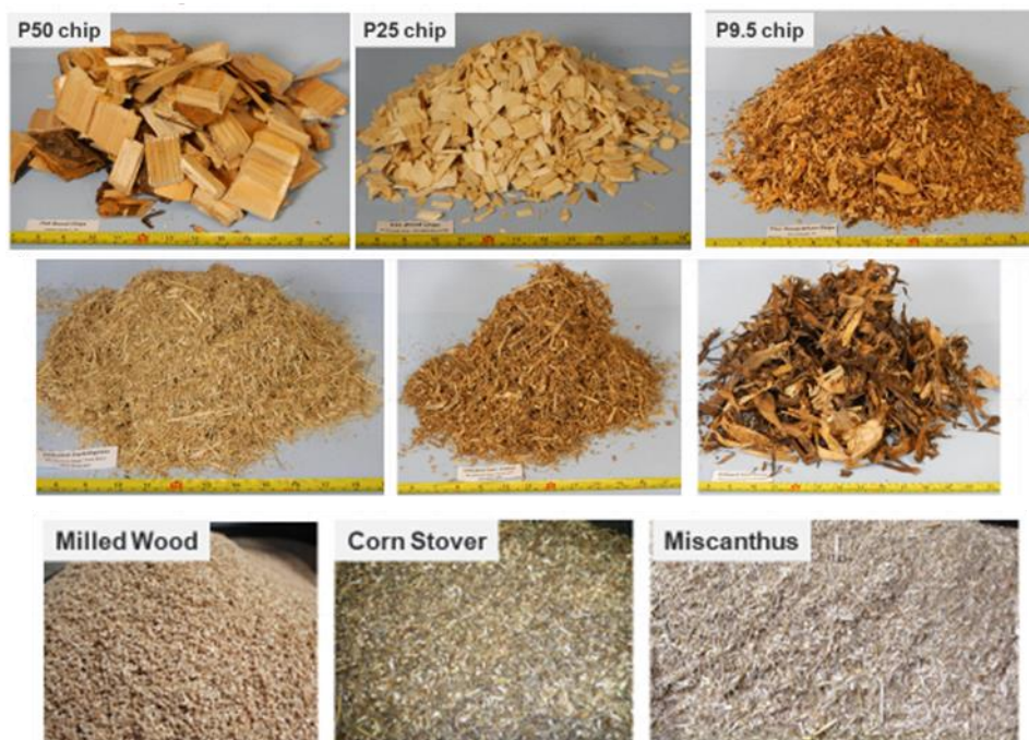
Figure 2. A selection of materials included in design considerations. Top) wood chips of various sizes and shapes; Middle) 1st stage processed herbaceous crop residues; Bottom) Reactor-ready feedstocks
