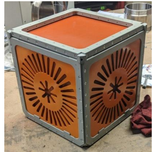
Figure 9. Biomass scale CTT sample holder with fixed rigid side plates installed
