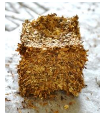
Figure 6. Shape of corn stover sample after HTC compression in PSU CTT
