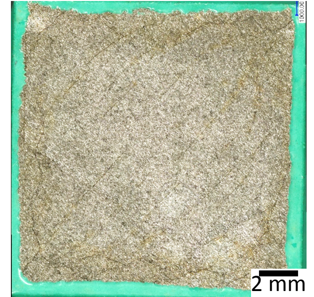
Annealed at 1200°C, 350 hrs. of immersion
