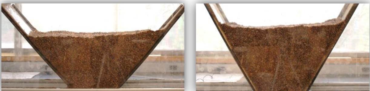
Figure 5 Typical experimental biomass flow set-up. Shown here are 45° and 60° hoppers filled with Corn stover 1 mm
