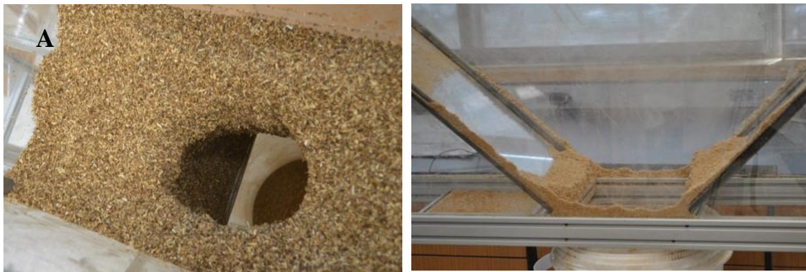
Figure 2 A. Typical corn stover hopper flow exhibiting a core-flow development and often resulting in a rat-hole and B. Typical Douglas fir hopper flow indicating a mass-flow
