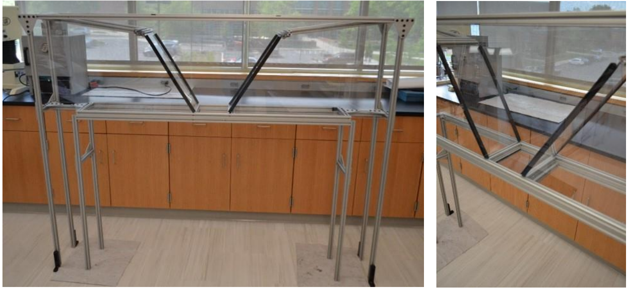
Figure 1 Lab-scale hopper with a variable wall angle and transparent sidewalls.
