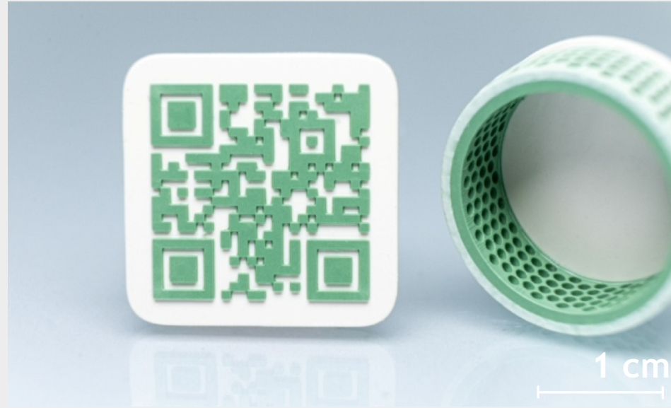
QR Code (coloured alumina) „green parts“
