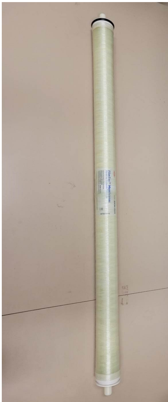
Figure 6.3. Photograph of BW30-2540-43 RO element.
