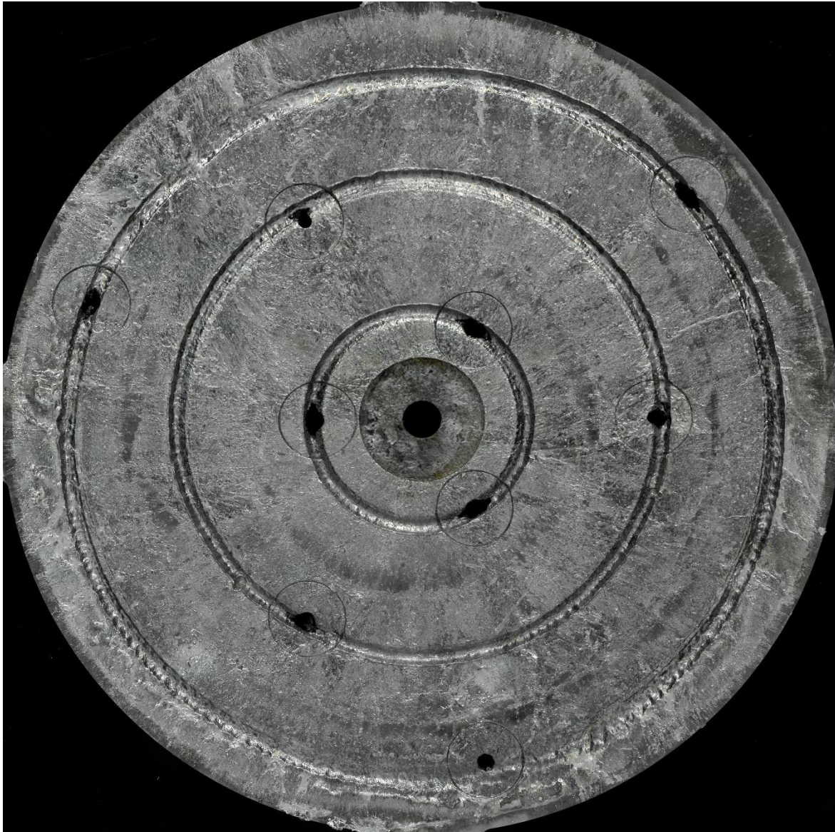
Figure 4-12. Top surface of the beam-stop on shot 4461 showing uniform burn pattern.
