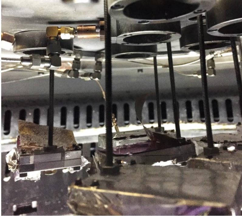
Figure 4-18. Photo of top surface of wedges showing damage from pinhole spall debris.
