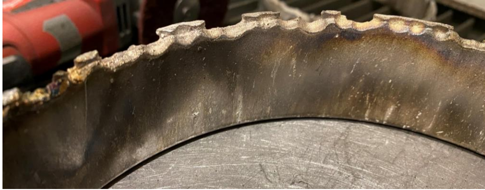
Figure 5-13. A photograph of the lower middle anode tip after a shot with significant beam steering off the middle cathode. The regularly spaced damage is a result of pinched beam strikes and was used to estimate the number of pinches per circumferential length of the cathode.
