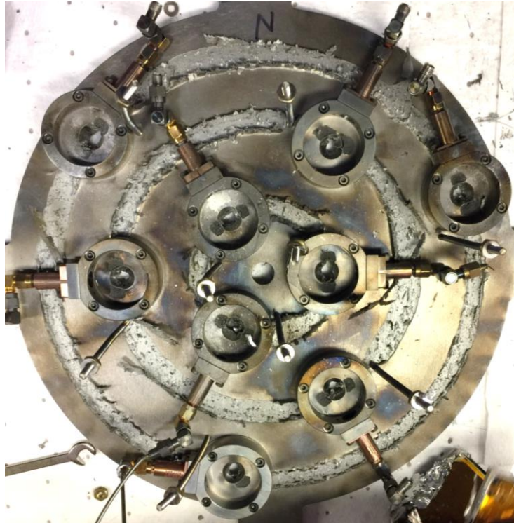
Figure 4-11. Bottom of the beam-stop for shot 4461 showing uniform spall pattern for all cathodes.
