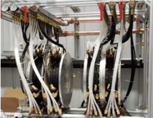
Fig. 10. An image of the Helmholtz coil component magnetic field testing facility currently under construction.
