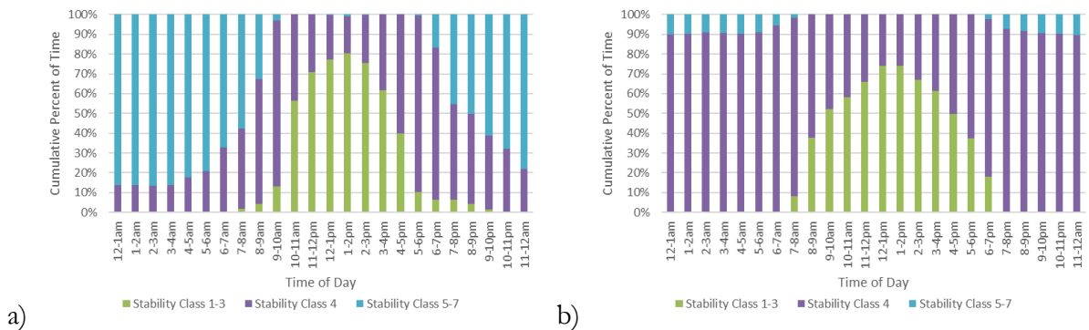
Figure 5-8. Stability class distribution as a function of time of day for the a) NAM12, and b) WRF27 data sets for Site D
