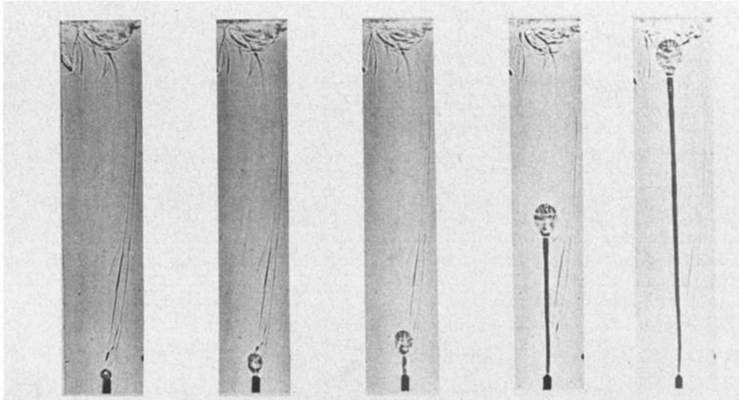
Buoyant rising of a less viscous fluid within a more viscous fluid ( $\mu_2/\mu_1 = 6000$ )
