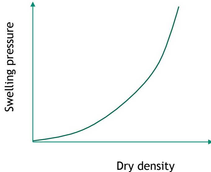
If gas migrates through channeling, the gas saturation degree would be  $\sim L_1 / (L_1 + L_2)$ , which is relatively small and determined by the swelling pressure curve.
