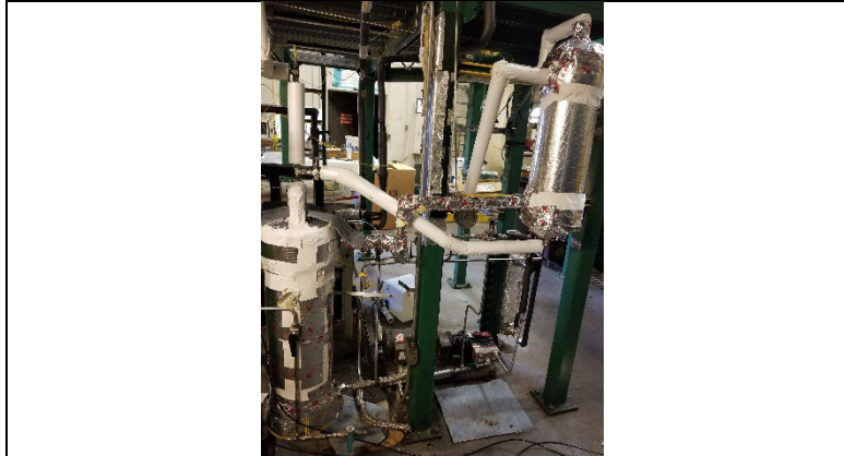
Exhibits 6.1.3. Picture of insulated heat exchangers for split flow configuration in 0.1 MWth unit.
