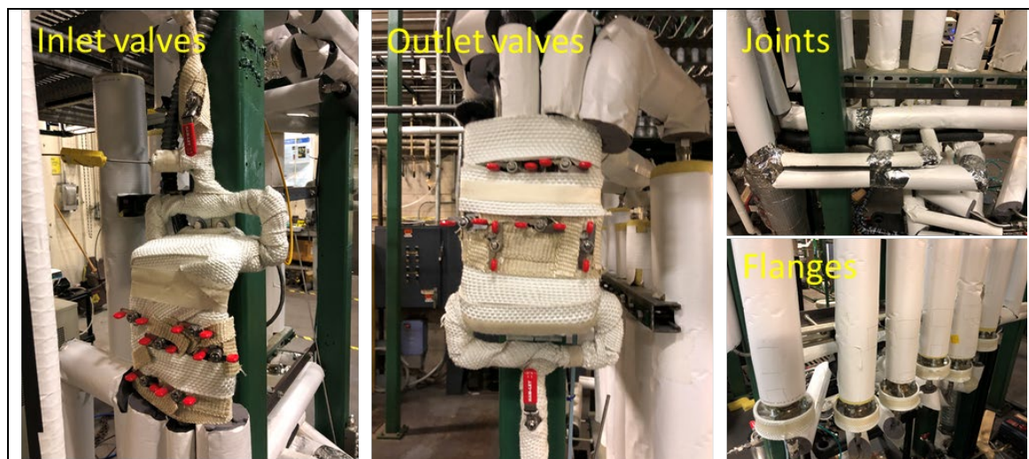
Exhibit 6.2.8. Six MPT NaY membrane bundles installed in the 0.1 MWth bench unit.
