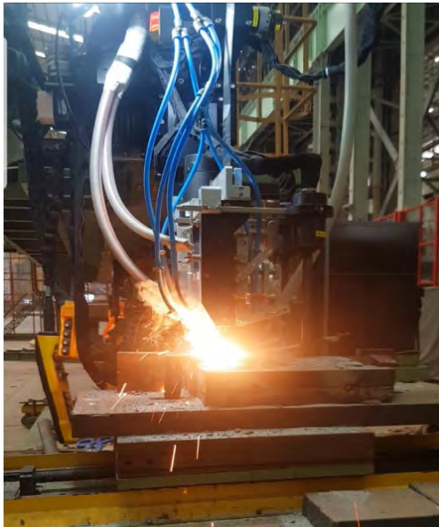
Automated cladding machine at Doosan
