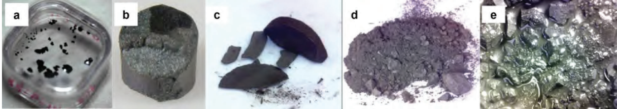
Figure 8: UN degradation under hydrolysis; a) UN pellet following static autoclave testing in DI water at 300 °C/10 MPa for 48 hours (modified from Nelson et al. ) [13], b) UN pellet after static auto testing at 300 °C/16 MPa for 30 minutes (modified from Watkins et al. ) [14], c) UN after hydrolysis in steam at 340 °C for 105 minutes, d) UN after hydrolysis in steam at 425 °C for 300 minutes (modified from Jolkkonen et al. ) [68], and e) UN after static autoclave corrosion at 300 °C, no time duration given (modified from Malkki) [76].
