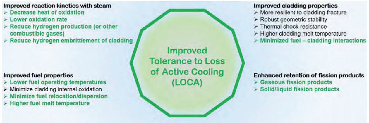
Figure 1: Primary attributes of accident tolerant fuels associated with fuel behavior and cladding at high temperatures. Modified from Carmack [32].
