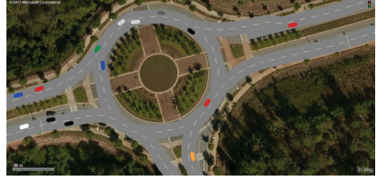
Fig. 4. A portion of vehicular traffic simulation with PTV VISSIM at the neighborhood of CU-ICAR.
