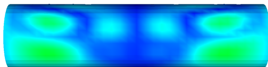
Figure 11-16. – Wet Modes Results. The mode shapes from wet modes can be visualized like any other Eigen solution case.
