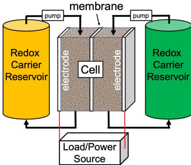
Redox flow batteries (RFB's) could be used to store energy from intermittent energy generation sources such as, wind and solar energy
