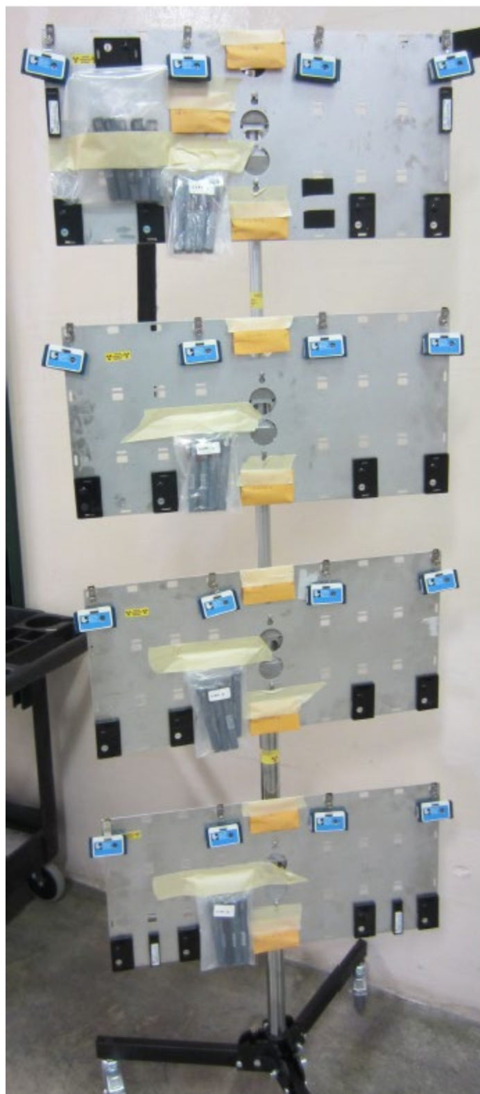
Figure 2. Dosimetry placed on aluminum plates on a rolling stand.
