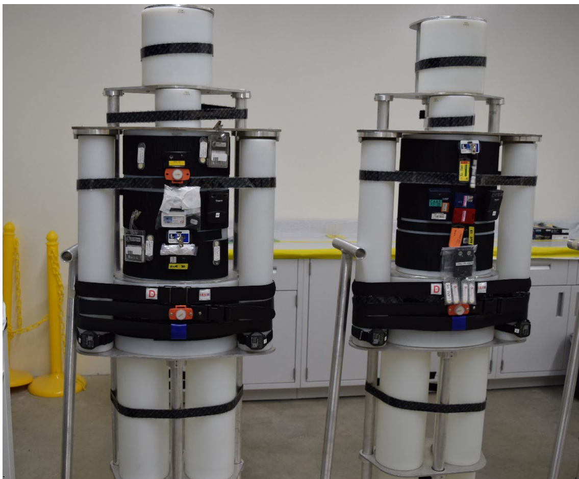
Figure 1. BOMAB on stand with dosimetry placed on front and backside.
