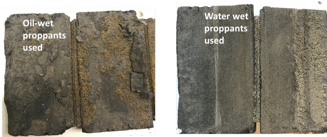
Figure 5.36 Fracture face of sample C3 after testing (Left) and fracture face of sample C7 after testing (right). The face of C3 showed significant damage compared to C7.
