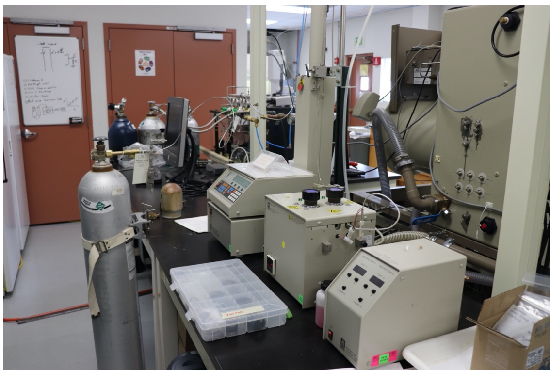
Figure 6.1 LANL Supercritical Fluid Extraction Facility. The system is comprised of a ISCO Type 260D syringe pump and controller system (SFX220) an extraction chamber or P-T vessel and a capillary tube restrictor heating system.
