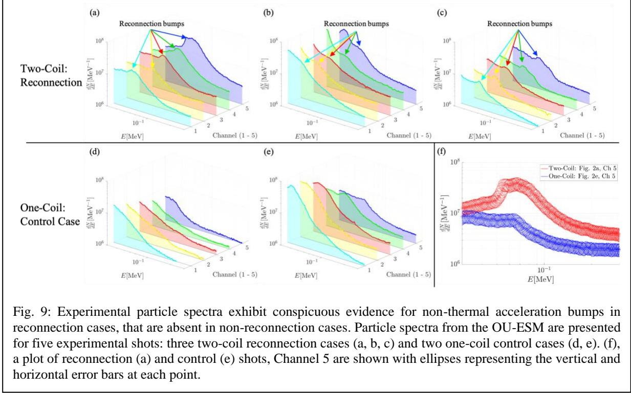
Fig. 9: Experimental particle spectra exhibit conspicuous evidence for non-thermal acceleration bumps in reconnection cases, that are absent in non-reconnection cases. Particle spectra from the OU-ESM are presented for five experimental shots: three two-coil reconnection cases (a, b, c) and two one-coil control cases (d, e). (f), a plot of reconnection (a) and control (e) shots, Channel 5 are shown with ellipses representing the vertical and horizontal error bars at each point.
