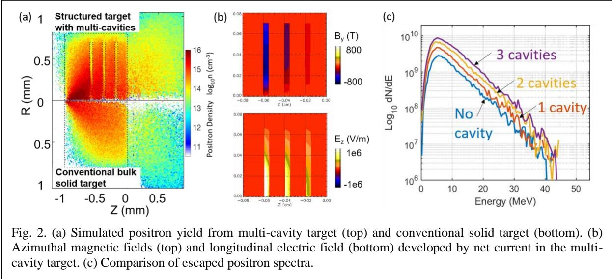
Fig. 2. (a) Simulated positron yield from multi-cavity target (top) and conventional solid target (bottom). (b) Azimuthal magnetic fields (top) and longitudinal electric field (bottom) developed by net current in the multi-cavity target. (c) Comparison of escaped positron spectra.
