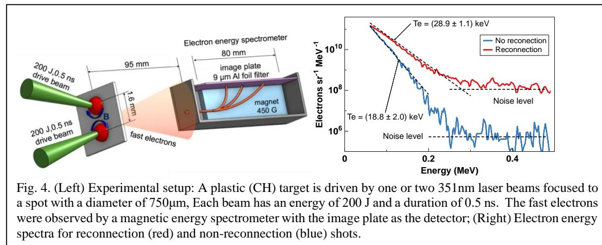
Fig. 4. (Left) Experimental setup: A plastic (CH) target is driven by one or two 351 nm laser beams focused to a spot with a diameter of 750 μm. Each beam has an energy of 200 J and a duration of 0.5 ns. The fast electrons were observed by a magnetic energy spectrometer with the image plate as the detector; (Right) Electron energy spectra for reconnection (red) and non-reconnection (blue) shots.
