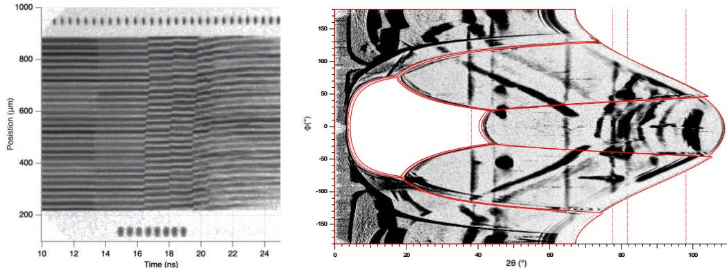
Fig. 10: Example of VISAR (left) and XRD (right) data obtained from 50  $\mu\text{m}$  thick Synthetic Uranus mixture at  $\sim 280$  GPa and  $\sim 2300$  K on OMEGA EP.
