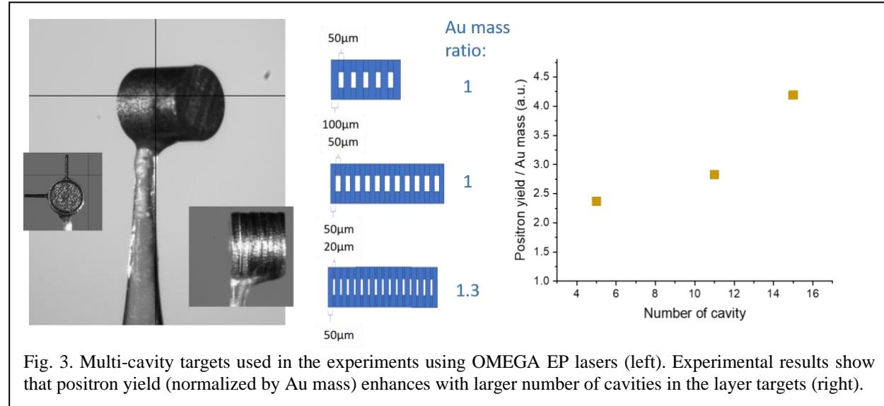
Fig. 3. Multi-cavity targets used in the experiments using OMEGA EP lasers (left). Experimental results show that positron yield (normalized by Au mass) enhances with larger number of cavities in the layer targets (right).
