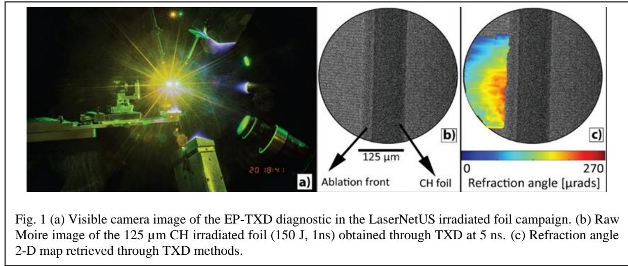
Fig. 1 (a) Visible camera image of the EP-TXD diagnostic in the LaserNetUS irradiated foil campaign. (b) Raw Moire image of the 125  $\mu$ m CH irradiated foil (150 J, 1ns) obtained through TXD at 5 ns. (c) Refraction angle 2-D map retrieved through TXD methods.
