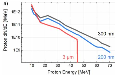
Fig. 7. Comparison of measured proton energy spectra. Proton results from the thin targets (300 nm and 200 nm) with >2 ps pulse show higher proton yield than the 3  $\mu$ m thick target case.
