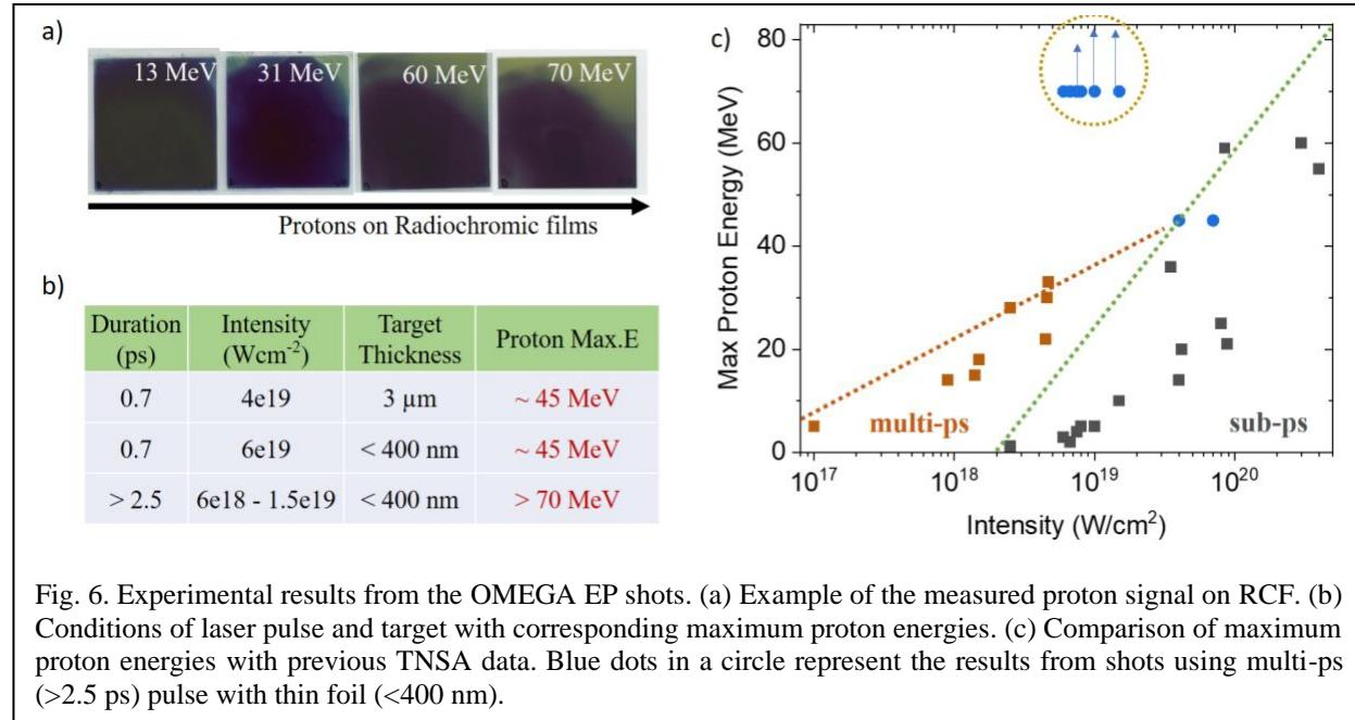
Fig. 6. Experimental results from the OMEGA EP shots. (a) Example of the measured proton signal on RCF. (b) Conditions of laser pulse and target with corresponding maximum proton energies. (c) Comparison of maximum proton energies with previous TNSA data. Blue dots in a circle represent the results from shots using multi-ps (>2.5 ps) pulse with thin foil (<400 nm).
