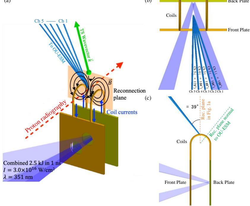
Fig. 8: Experimental setup of low- $\beta$ , magnetically driven reconnection using laser-powered capacitor coils. (a) The capacitor-coil target is driven by two long-pulse lasers, passing through the front holes and irradiating the back plate. (b) and (c) are the top-down view and the side view of the target along with the OU-ESM channel orientation.
