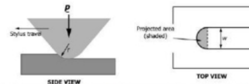
NOTE 1—The contact of the stylus is assumed to produce a semi-circular projected area when viewed from the top.
