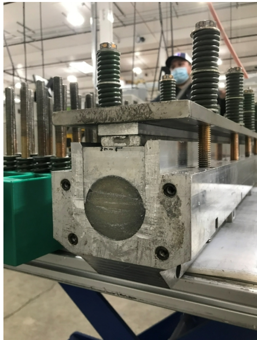
Quarter Nano direct draw (1 st draw) – compressed into fusing die
