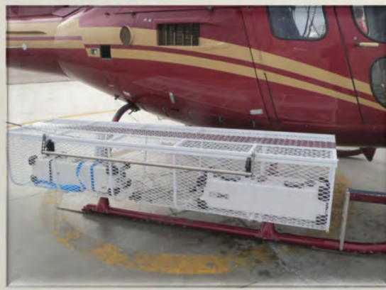
Mirion detectors in the external basket mounted to the helicopter skids utilized by French IRSN
