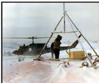
A microwave ranging transponder unit is placed under a landmark. The distance limitations of the units meant constant movement was necessary as the search moved along the footprint.
