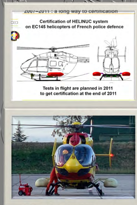
Custom designed, built, and certified detector pods utilized by French CEA
