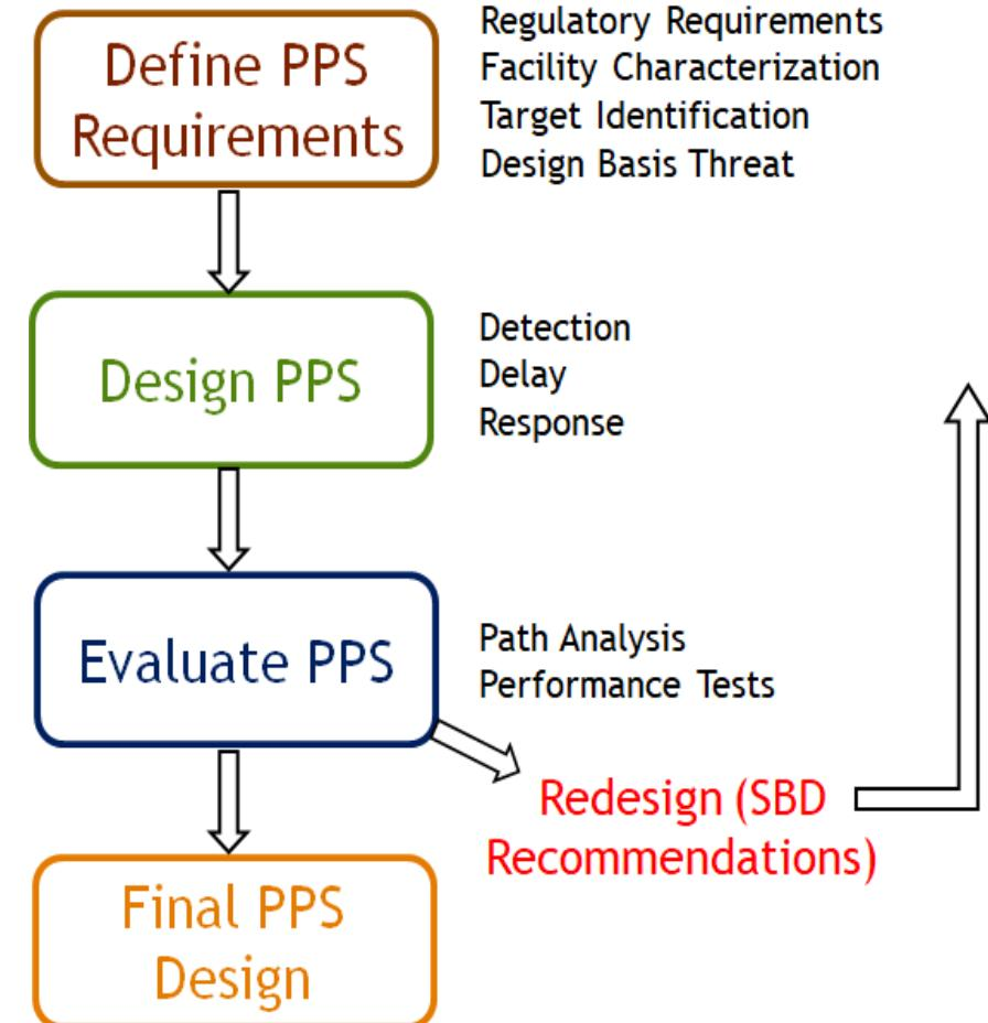
The Design Evaluation Process Outline (DEPO) is a systems engineering method that has been applied to nuclear security since the 1970's. DEPO is a performance-based methodology to design and evaluate physical protection systems (PPS) against the threat of unauthorized removal of nuclear materials or radiological sabotage.
