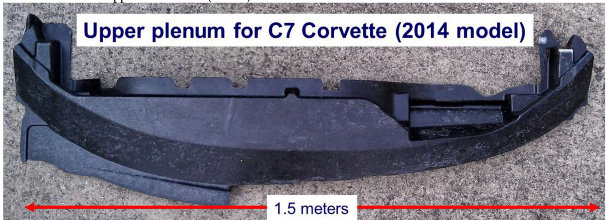
Figure 1. Upper plenum for C7 Corvette. The recycled carbon fiber preform was made using the CCI large 3-DEP® machine. The composite part was molded by the Molded Fiber Glass Company (Ashtabula, OH) using liquid compression molding in a matched metal tool.
