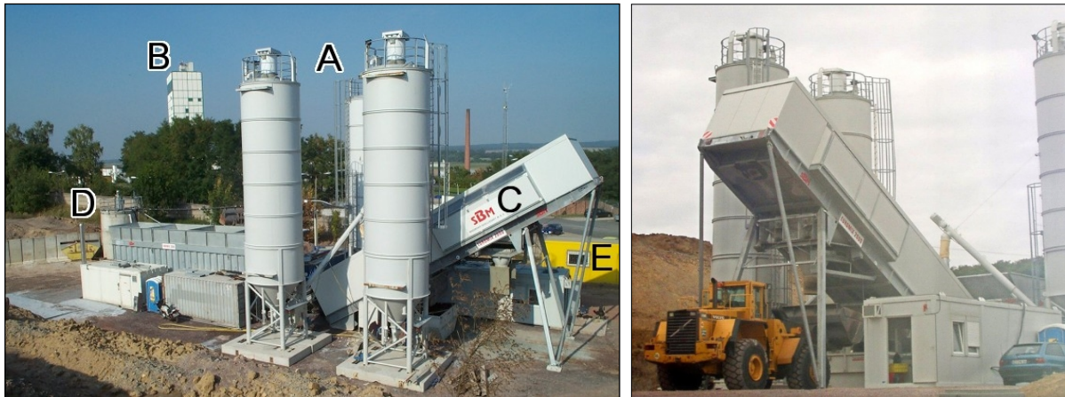
Figure 4-8: Mixing plant for salt concrete on surface (A: silos for the storage of cement and fly ash, B: shaft Bartensleben, C: concrete batch mixer, D: tank for salination of the mixing solution, E: container for quality control) (Fischer et al., 2004)
