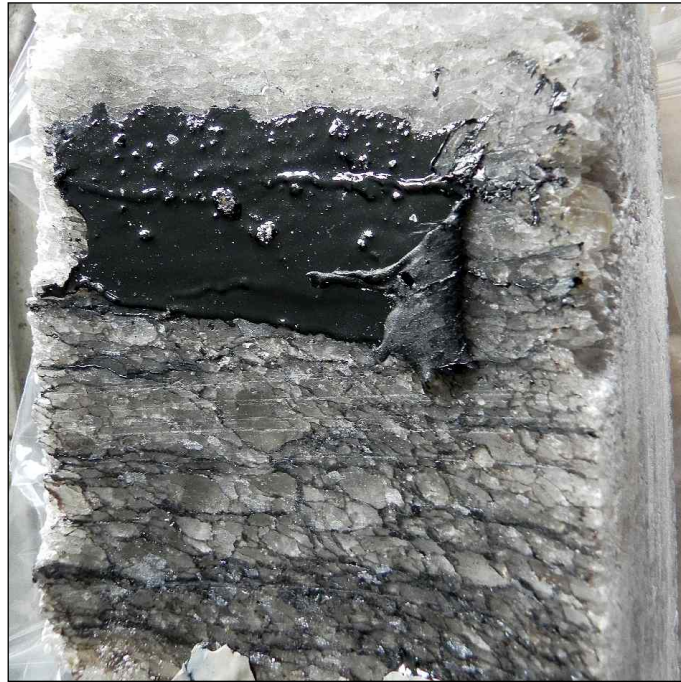
Figure 2-17: Image of sample from the borehole edge after removal of the test (Kudla et al., 2021)
