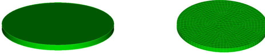
Figure 4-7. – PZT5A disc verification problem
