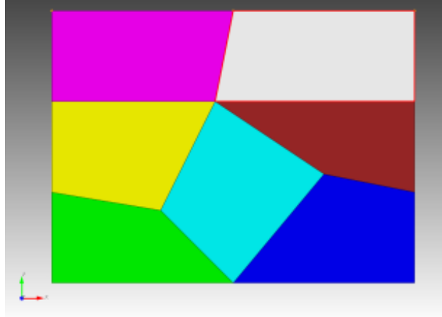
Figure 9-14. – Patch Test Geometry
