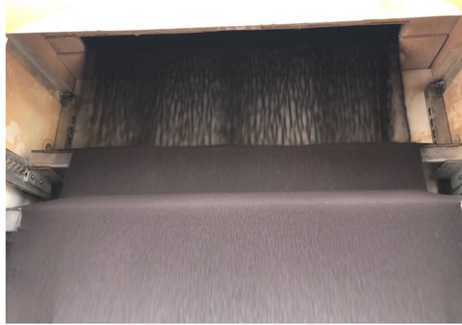
Figure 29. Left: Multi-cavity molten-salt receiver at Khi Solar One . Right: Particles falling over catch-and-release troughs in a cavity receiver during testing at Sandia.
