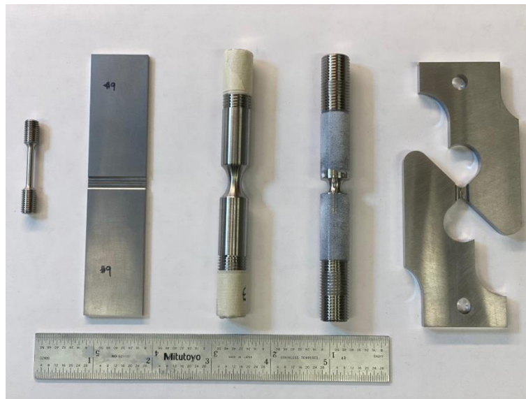
Figure 1. The test specimens are left to right: standard tensile (R5), flat groove, 9 mm notch, 3 mm notch, and shear specimens
