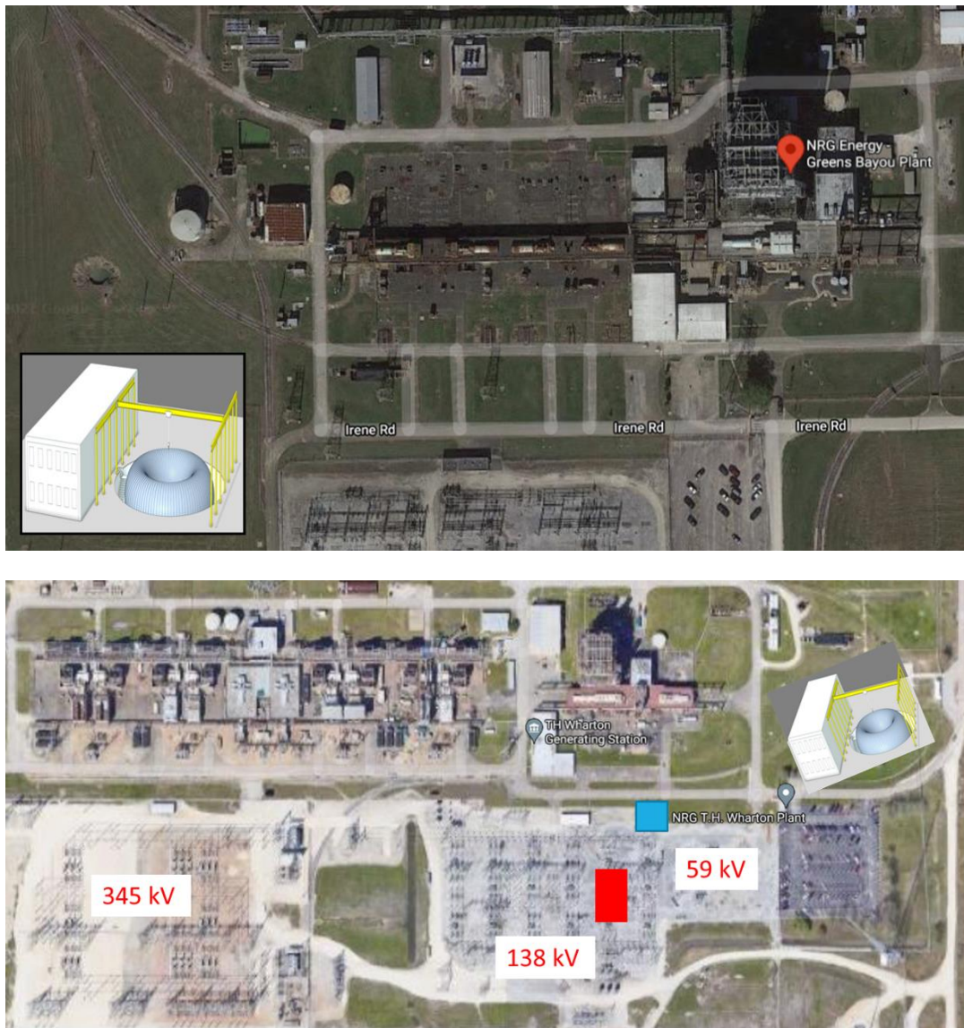
Figure 18 Site plans and SMES integration for NRG Greens Bayou (top) and NRG TH Wharton (bottom)
