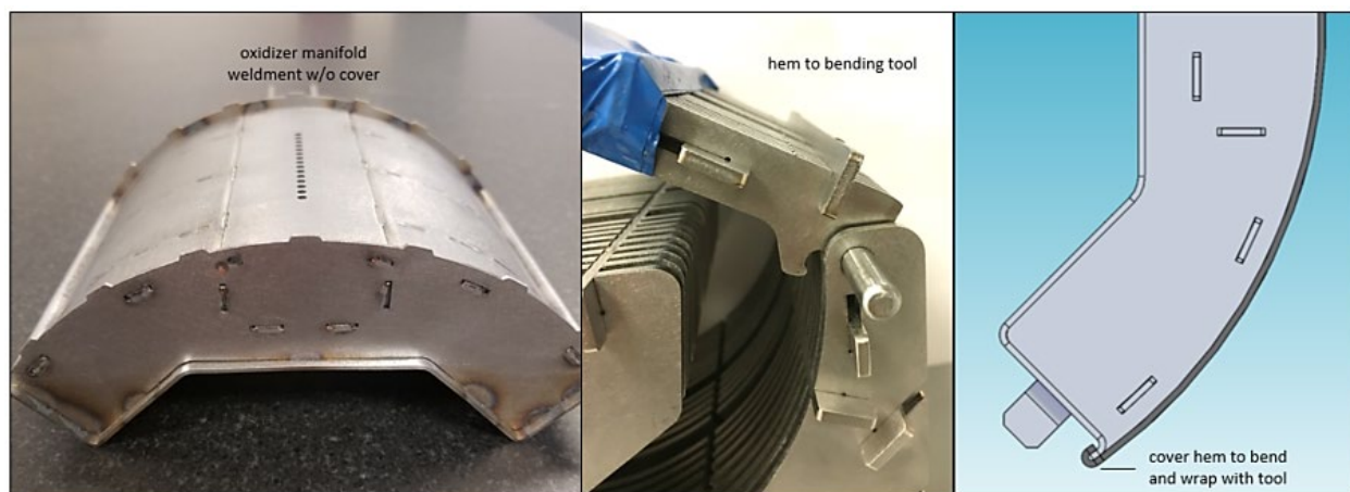
Figure 3.3-5 Fabrication of Oxidizer Manifold
