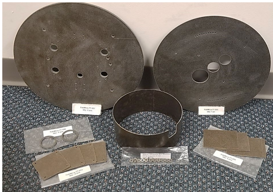
Figure 3.3-13 Fabricated Mica Components
