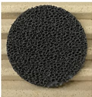
Figure 3.1-34 High porosity substrate, 1" diameter (left). Relationship between cumulative weight and number of coatings. After 1 st coating, the coated sample was dried at 120°C for 30 minutes. After the second coating, the sample was calcined at 550°C for three hours. Sample 1, 2, and 3 were from the same batch of the porous substrate. Sample 1 was uncoated porous substrate (not shown).
