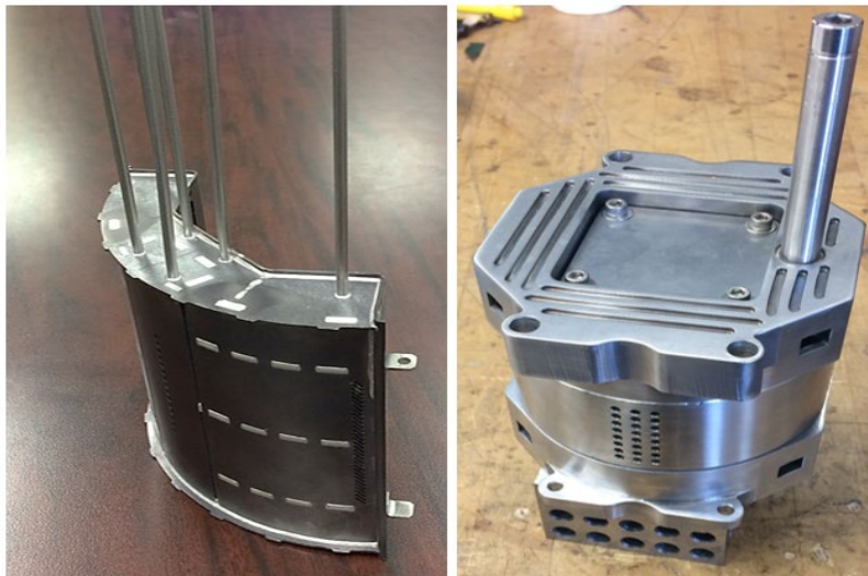
Figure 4.1-7 Mock Stack Components – Oxidizer Manifold (left); Core and End Plates (right)
