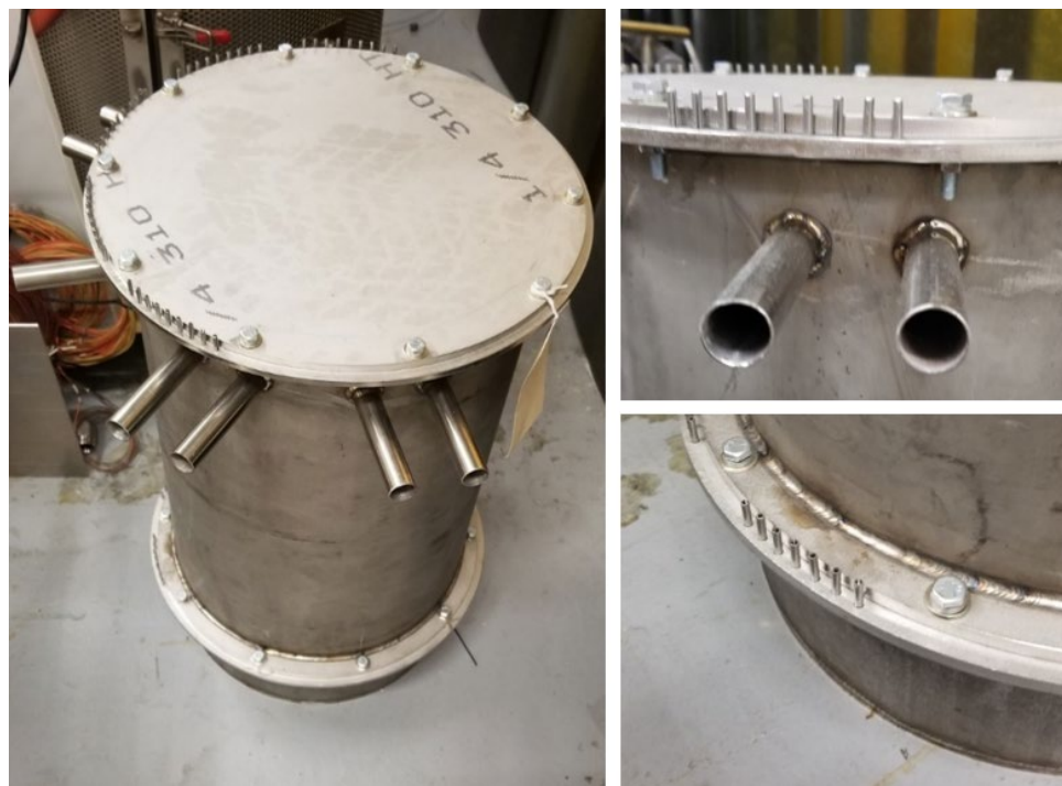
Figure 4.1-5 Stack Containment Vessel Housing Assembly – as built
