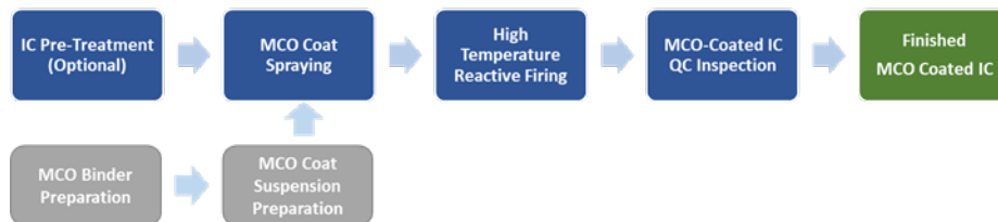
Figure 5.1-5 FCE In-house MCO Coating Interconnect (IC) Process Flow
