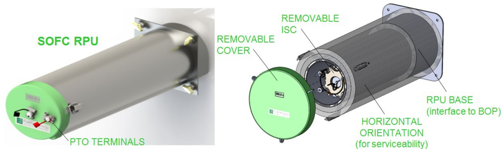
Figure 3.1-51 Layout of the RPU during CAD Design Activities
