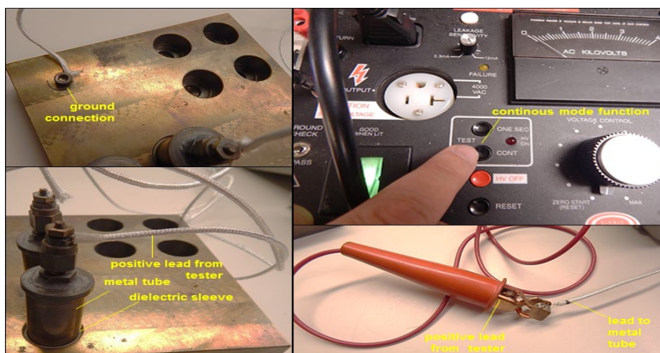
Figure 3.1-47 HIPOT Test
