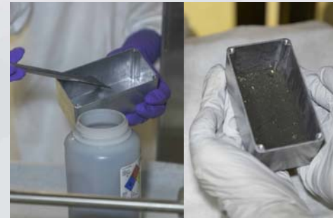
Material loading process and filled source container
