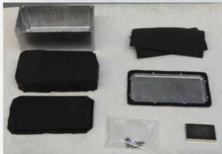
Source materials comprising project box, gasket, closed cell foams and rare earth magnets
