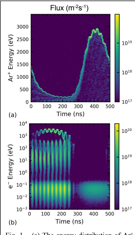
Fig. 1 – (a) The energy distribution of  $\text{Ar}^+$  ions and (b) electrons reaching the lower electrode as a function of time in the low frequency cycle.
