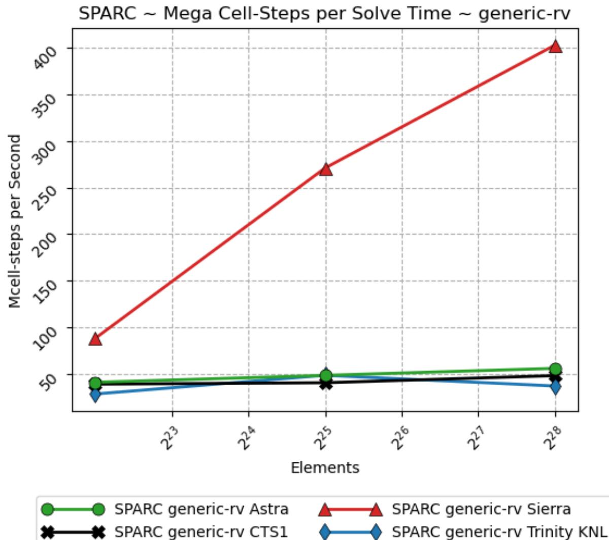
Throughput calculated from 64 node runs of R0, R1, R2 meshes.
