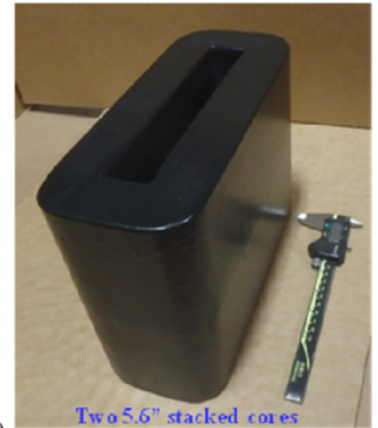
Figure 3: a) Full sized spool of 142mm (5.6") wide FT-3W weighing 500 kgs and b) Inductor core fabricated from the 142mm nanocrystalline FT-3W ribbon.
