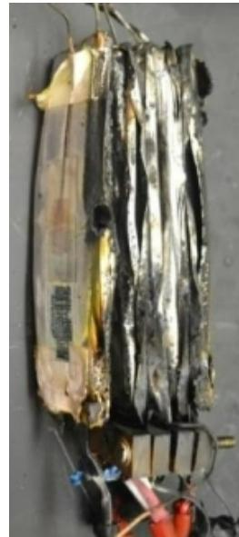
Short circuit simulated in first cell acts as boundary condition
