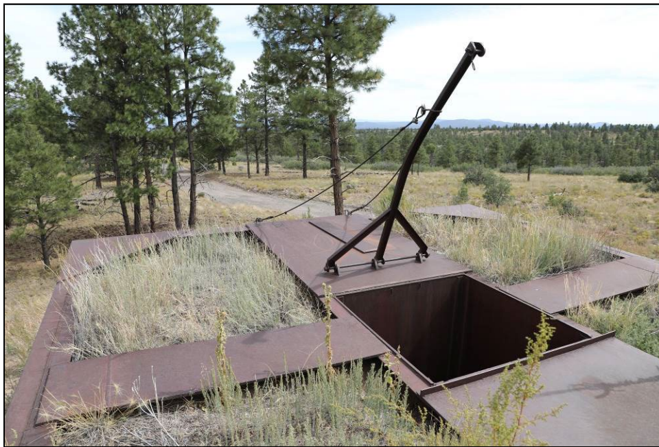
Figure 211. Test were lowered into the square hole using the adjacent boom.
