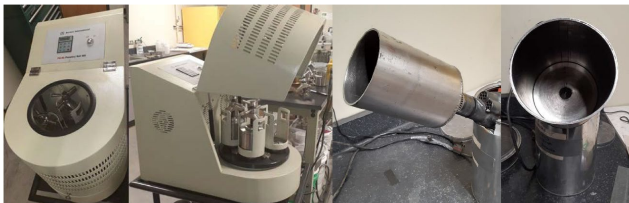
Figure 3-1 Image of Ball Mill Unit (left) and Pan Mixer (Right) for homogenizing and pelletizing sample
