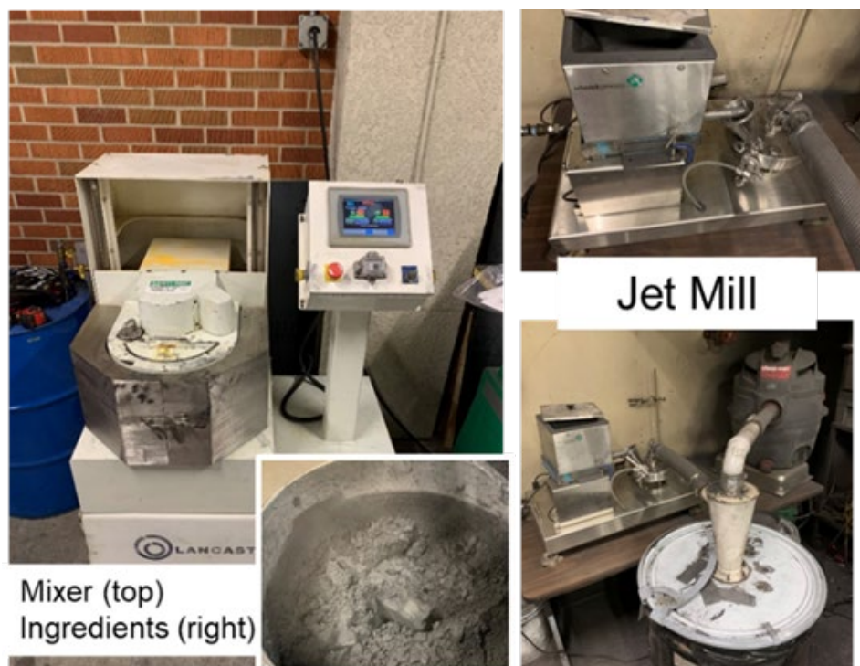
Figure 3-42 Lancaster K-1 mixer for preparing oxygen carrier formulations
