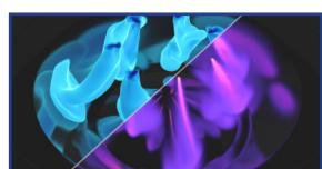
Predictive simulations of the complex incylinder processes of internal combustion engines that are being used to improve performance and decrease pollutant emissions. Credit: Kenny Gruchalla, National Renewable Energy Laboratory
