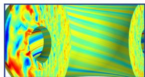
A visualization of deuterium-tritium density fluctuations in a tokamak driven by turbulence. Areas of red are representative of high density and areas of blue are representative of low density. Credit: Emily Belli, General Atomics
