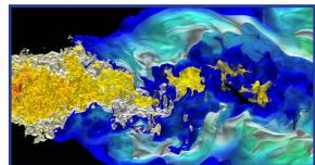
Direct numerical simulation reveals turbulent combustion of direct-injection processes in internal-combustion engines and provides an essential component for development of high-efficiency, low-emissions vehicles. Credit: Jacqueline Chen, Sandia National Laboratories
