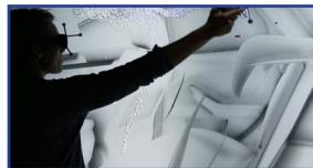
An engineer interactively exploring complex airflow inside an electric vehicle cabin by directly seeding particles in the flow. Credit: John De La Rosa, National Renewable Energy Laboratory
