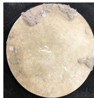
Figure 5. Impurities from commercial HMX as received not passing the 1 μm GF/B filter in the new glass thimble.
