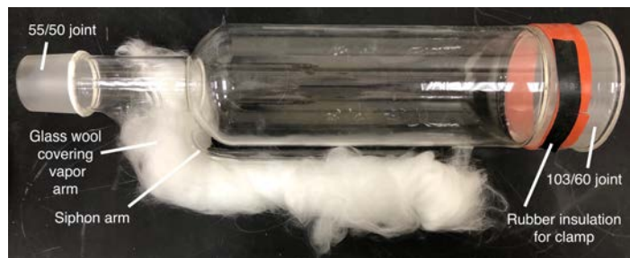
Figure 7. Soxhlet extractor design, with glass wool wrapped around vapor arm, PTFE rope around 55/50 joint, and rubber sleeve for clamp connection.
