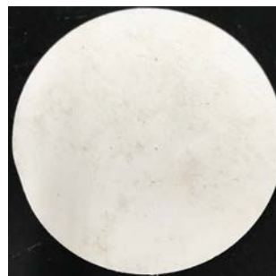
Figure 6. Impurities resulting from the 0.7 μm GF/F filter extraction of material previously extracted through a 1 μm GF/B filter.
