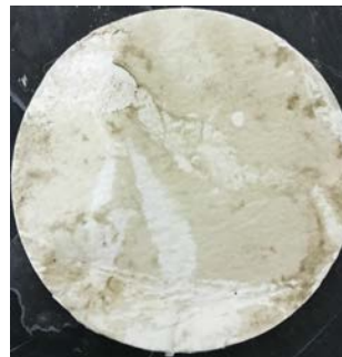
Figure 4. Impurities passing the cellulose thimble but caught on the 1 μm GF/B filter in the new glass thimble.
