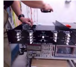
Assembling the broadband laser ranging diagnostics used in the Sierra Nevada SCEs
