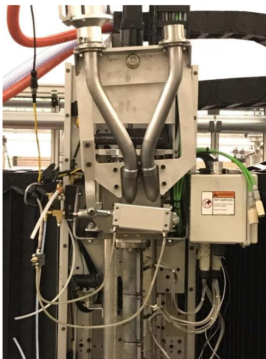
Figure 1: The newly installed dual-hopper system on the MDF's BAAM-B. This system enables in-situ material switching for MM and FGM large-scale printing of thermoplastics.
