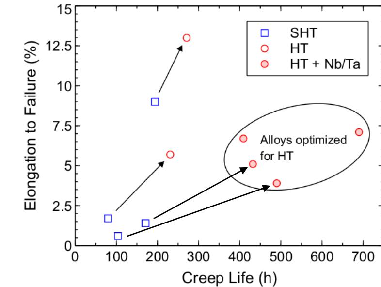
▲ Elongation to failure vs creep life following testing at 700°C / 70ksi.
