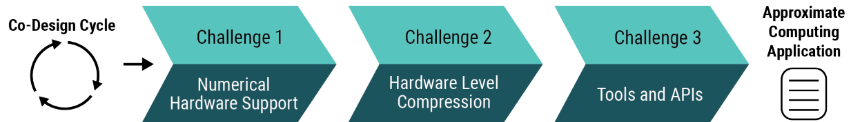
Figure 1: Overview of the challenges to co-design AC applications. The challenges include (1) hardware support for multiple levels of floating-point precision and new numerical representations, (2) hardware-level support for numerical compression, and (3) improved tools and compilers to apply multiple AC methods automatically.
