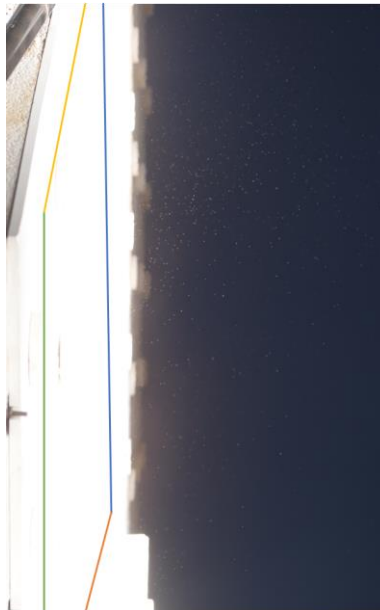
Figure 51. For the analysis, the image is adjusted so the flow of particles is to the positive side of the X-axis. The blue line denotes the top, the green line is the bottom, the orange line is the East side and the yellow line the West side of the FPR aperture.
