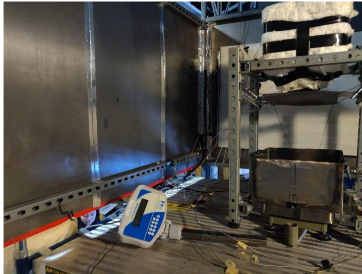
Figure 21. DAQ system wiring of SPR connects all thermocouples and digital scale to the central computers.
