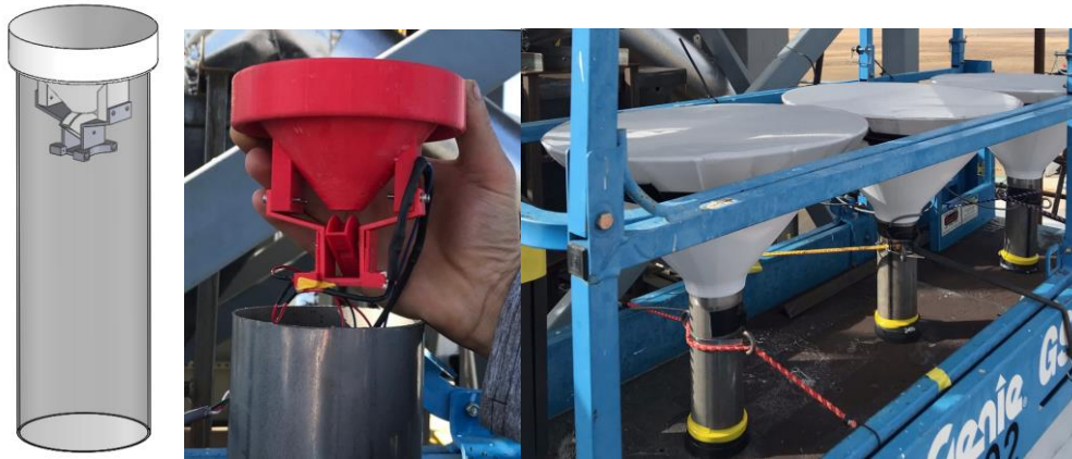
Figure 89: PLA Tipping Bucket Design, Preliminary Prototype and Full-Scale Setup.
