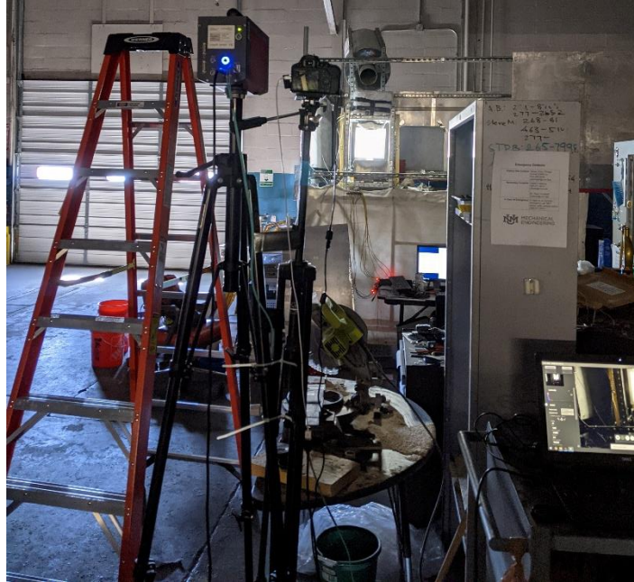
Figure 24. The IR and Nikon cameras mounted 5 meters away along with the laptop to capture both images and thermograms.
