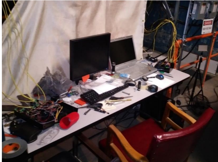
Figure 22. Two computers are used to monitor and record data from thermocouples, cameras, and digital scale.
