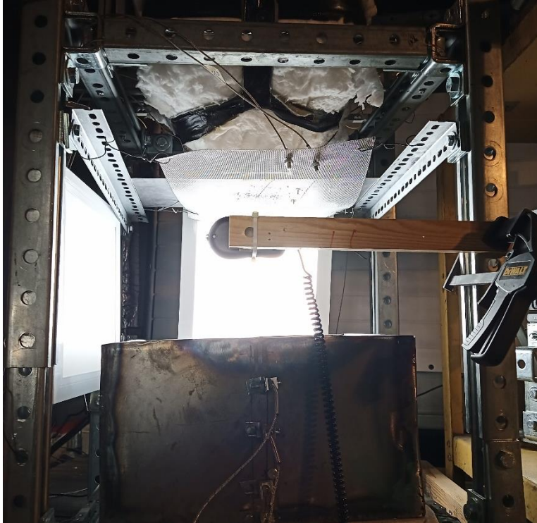
Figure 8. An LX1330B lux meter was used to estimate the opacity of the curtain. The lux meter was mounted in an arm and measurements were taken in 5 different positions.
