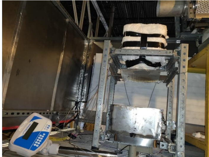
Figure 17. A \pm 0.5 g resolution scale is being used in place to track the weight change due to the particle flow.
