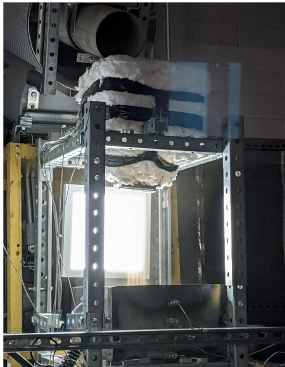
Figure 20. LED panel was installed to create contrast between the background and the particles.
