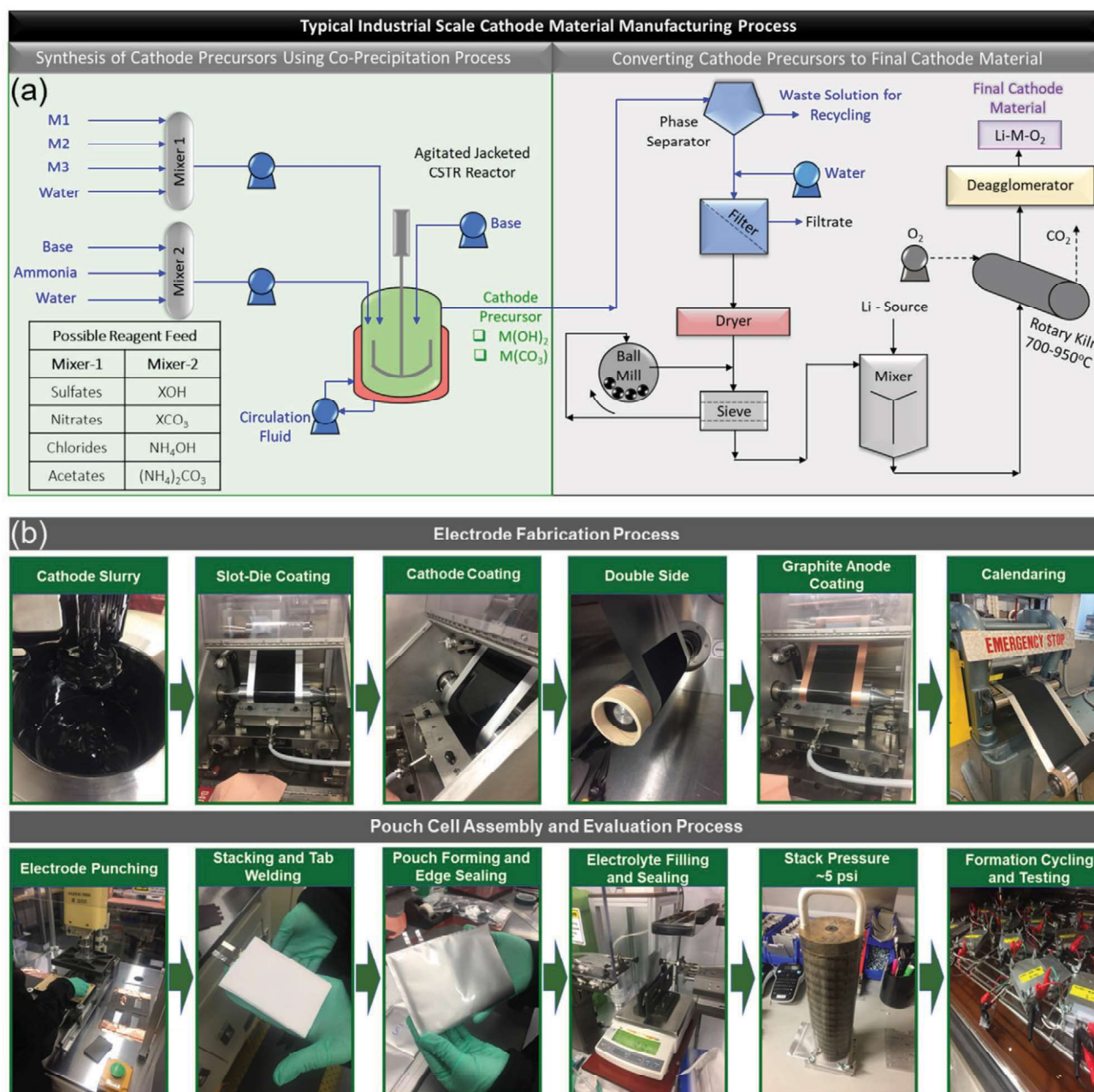
Figure 10. a) Schematic of an industrial scale cathode material manufacturing process and b) electrode coating protocols and cell fabrication techniques employed in commercial battery manufacturing. [48]
