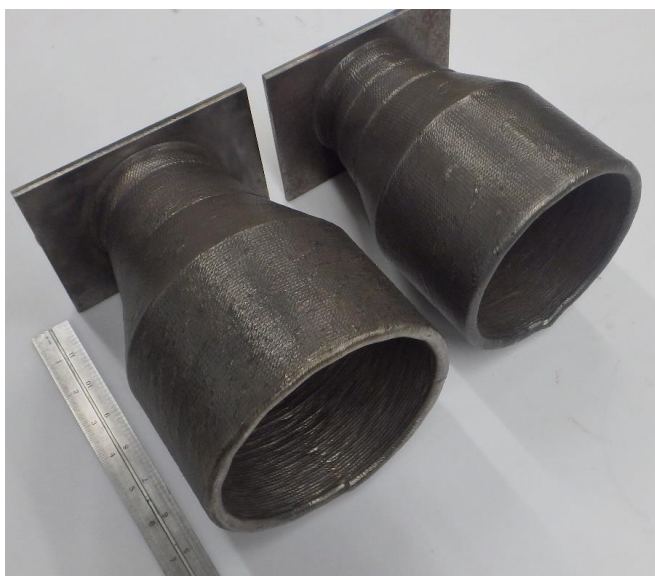
Figure 166. Variable diameter tube/pipe sections, deposited via WAAM using a high-strength low alloy steel. Shows feasibility of 3D printed components for power applications.
