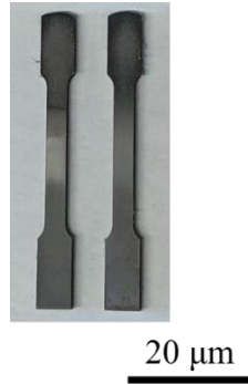
Figure 117. Tensile bars extracted from the 60 and 85 wt.% P91 builds for mechanical testing.
