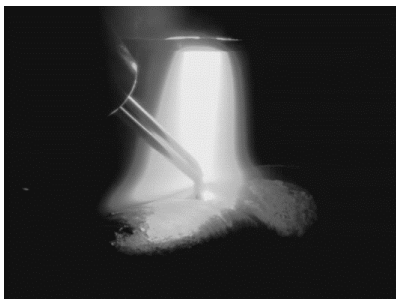
Figure 95. Image from the deposition process with twin-wire feed.
