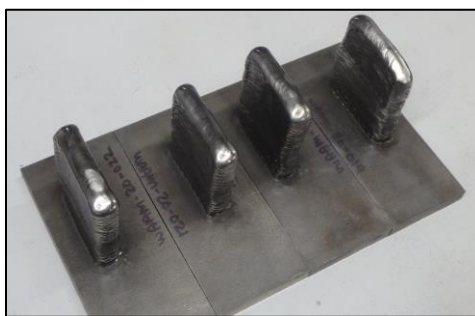
Figure 96. WAAM coupons with various material gradients/blends.
