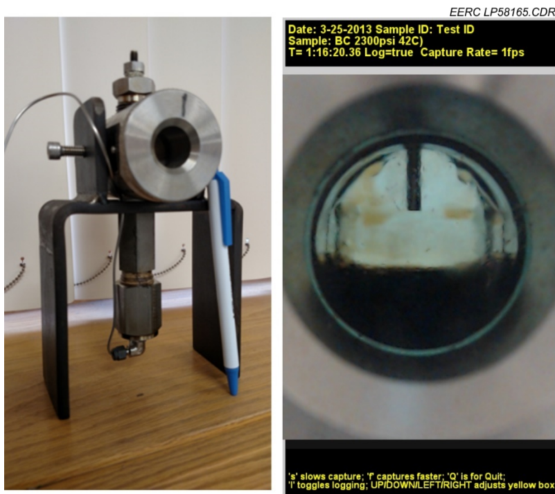
Figure 3. Test cell (left image) and cell with two fluid phases present (right image). The gas is percolated through a 10-mL (8-gram) oil column and equilibrated at reservoir temperature (23°F) and pressure (1500–5000 psi). The upper “miscible” phase is sampled while maintaining reservoir temperature and pressure. Dissolved HCs are collected and analyzed by GC/FID.
