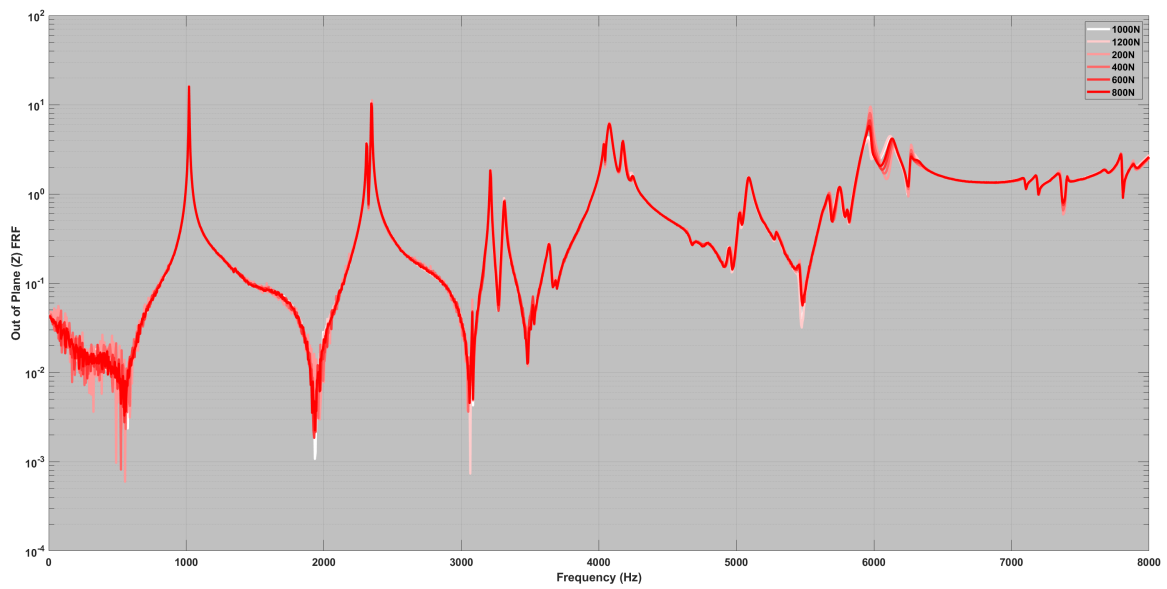
Figure 4-7. Nonlinear analysis of the bare resonant plate
