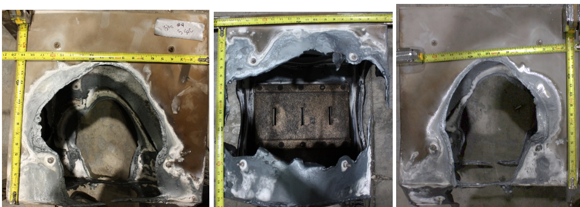
Fig. 87. Experiment OBMV4 enclosure breach (Left-to-right: Right side, back side, left side)
