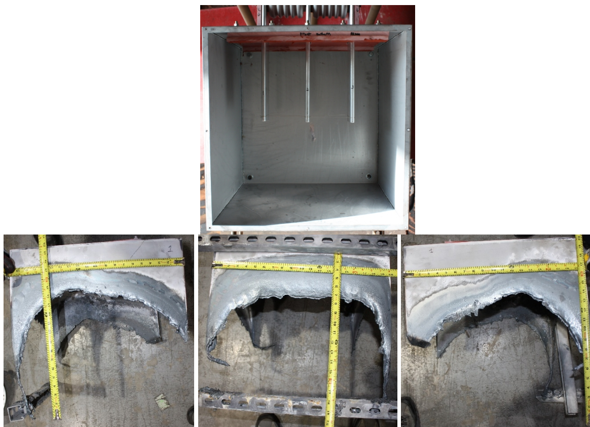
Fig. 98. Experiment OBMV01 pre-experiment (top) and post-experiment (bottom left – side, bottom center – back, bottom right - side). Phase sequence from left to right is C-B-A.
