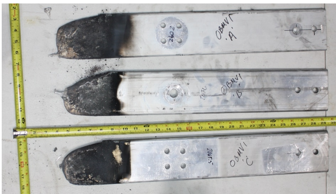
Fig. 99. Experiment OBMV1 electrode post-experiment
