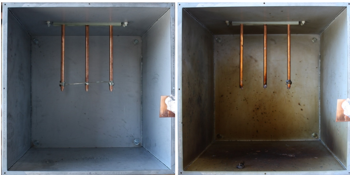
Fig. 28. Experiment OB01(a) Pre-experiment (left) and Post-experiment (right) electrodes. Phase sequence left-to-right (C-B-A)
