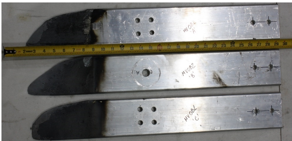
Fig. 107. Experiment OBMV2 aluminum electrodes post-experiment
