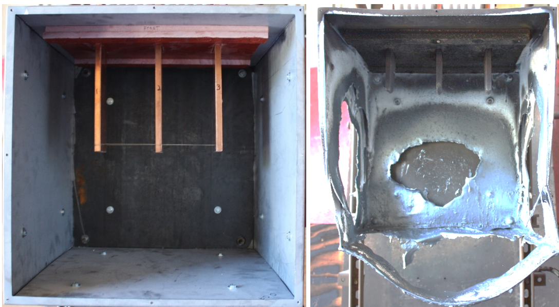
Fig. 86. Experiment OBMV04 pre-experiment (left) and post-experiment (right) electrodes. Phase sequence from left to right is C-B-A.
