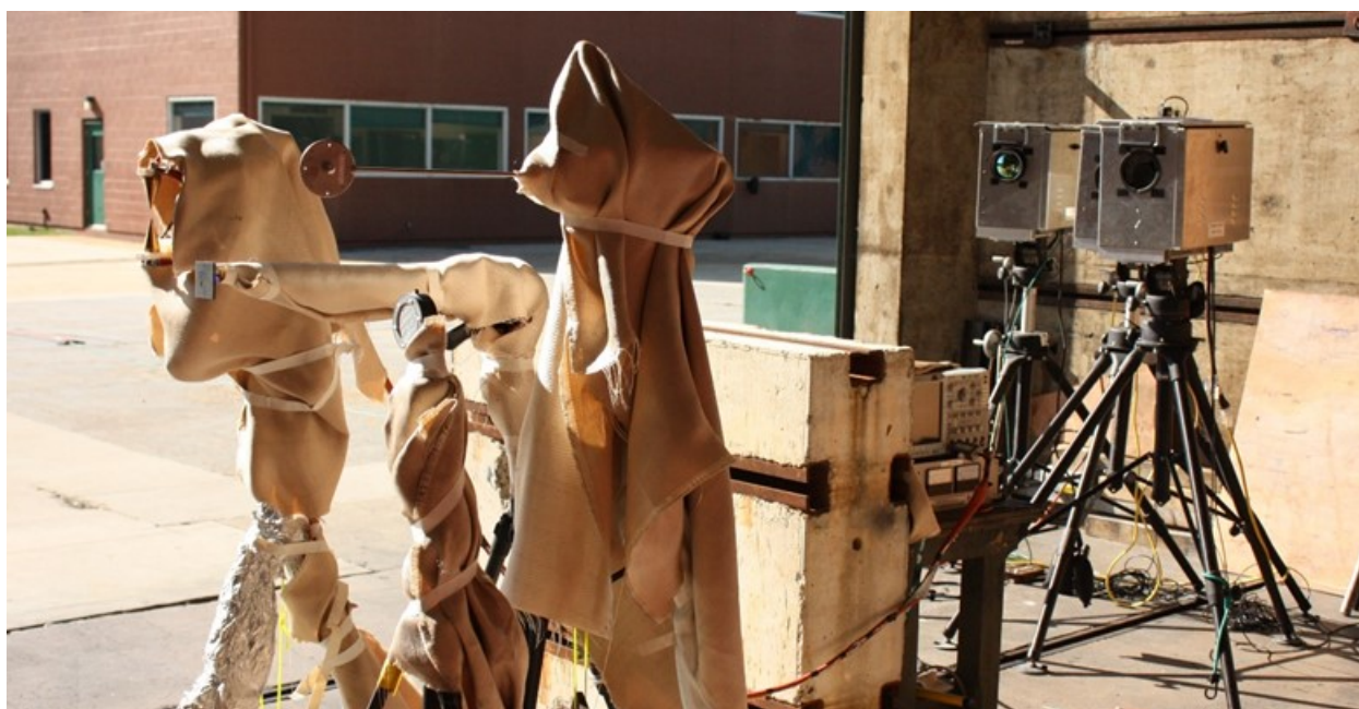
Fig. 6. Instrumentation cluster covered with heat resisting fabric for protection during experiments (from Left-to-right, air breakdown, radiometer, d-dot, air conductivity, high speed IR and visible videography)
