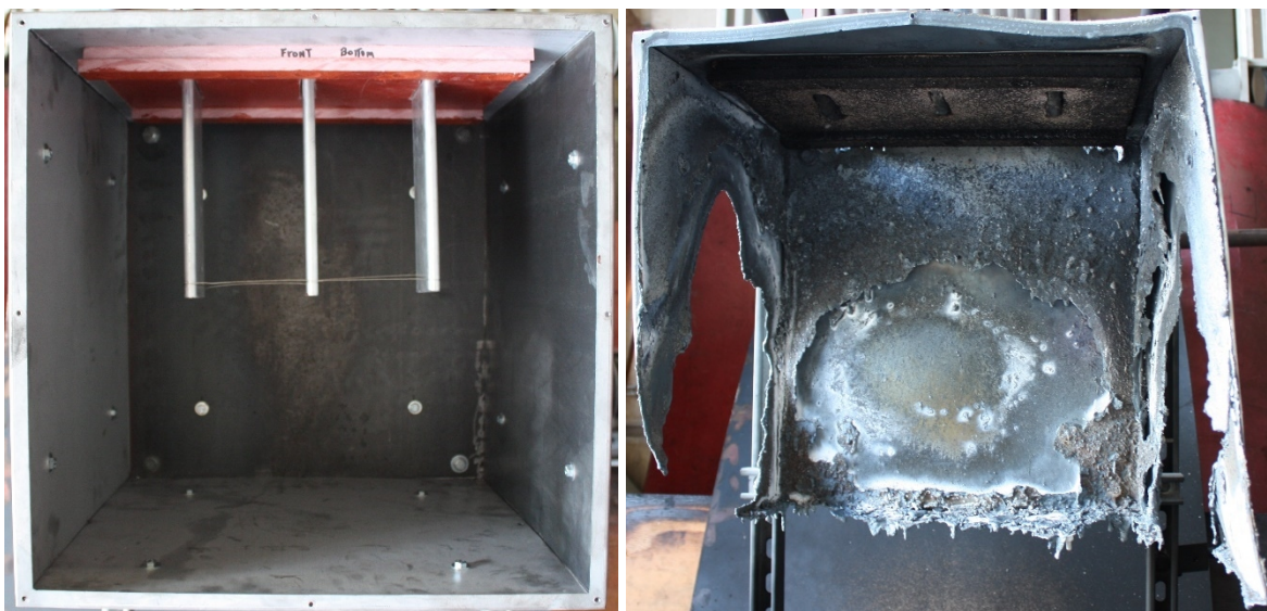
Fig. 115. Experiment OBMV03 pre-experiment (left) and post-experiment (right) electrodes. Phase sequence left to right is C-B-A.
