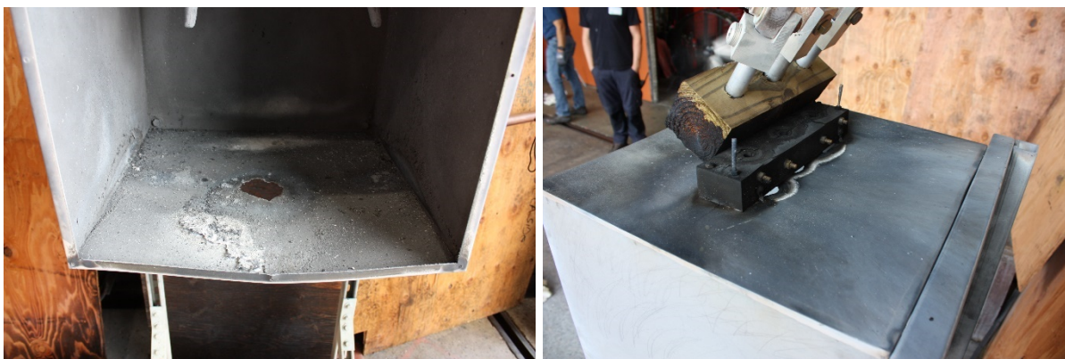
Fig. 75. Experiment OB08 enclosure breach (Left –bottom and sides; Right – rear top).
