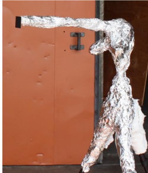
Fig. 10. Radiometer apparatus in its thermal protected configuration
