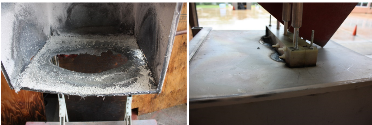
Fig. 69. Experiment OB07 enclosure breach (Left – bottom and sides; Right – rear top side).
