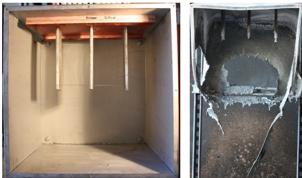
Fig. 123. Experiment OBMV06 pre-experiment (left) and post-experiment (right) electrodes. Phase sequence from left to right is C-B-A.
