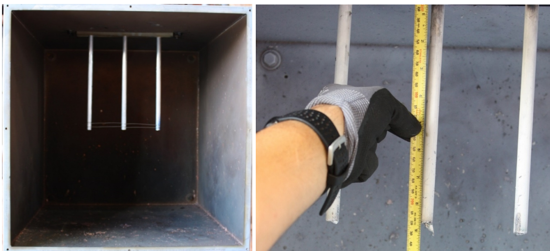
Fig. 59. Experiment OB05 pre-experiment (left) and post-experiment (right) electrodes. Phase sequence from left-to-right is C-B-A.
