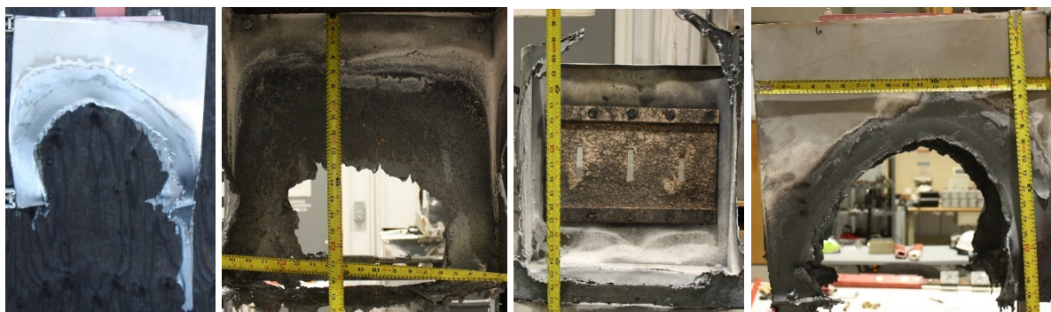
Fig. 124. Experiment OBMV06 enclosure breach (Left-to-right: left side, back side, bottom side, and right side)
