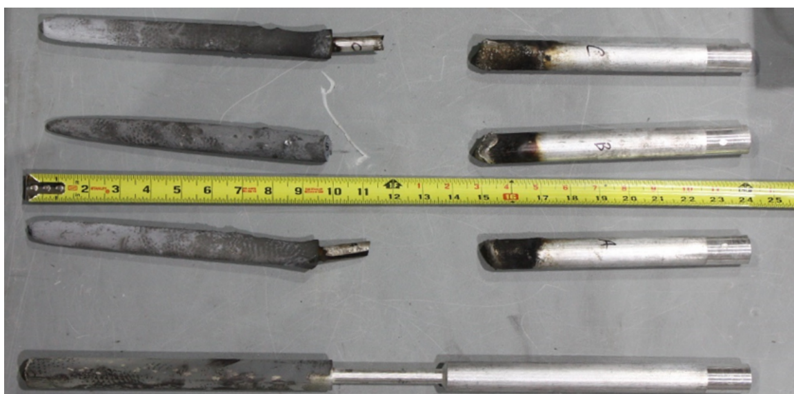
Fig. 76. Experiments OB08 aluminum electrodes post-experiment top three. (Bottom electrode is from other another experiment and included for comparison)
