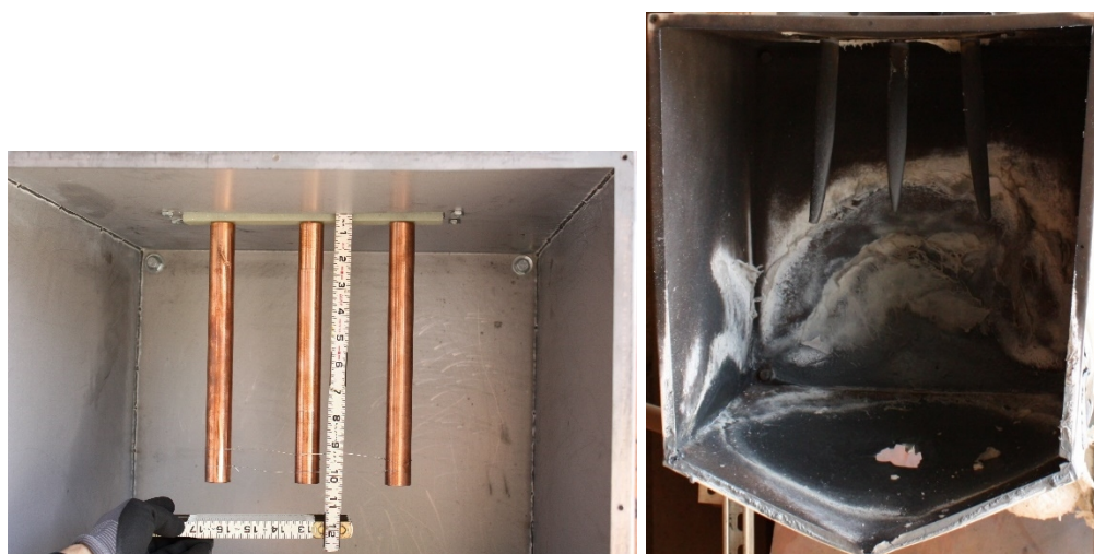
Fig. 48. Experiment OB04 pre-experiment (left) and post-experiment (right) electrodes. Phase sequence from left to right is C-B-A
