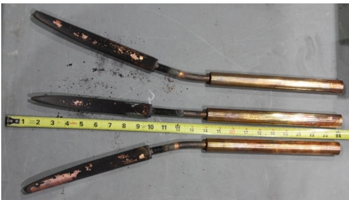
Fig. 50. Experiment OB04 electrode deflection post-experiment
