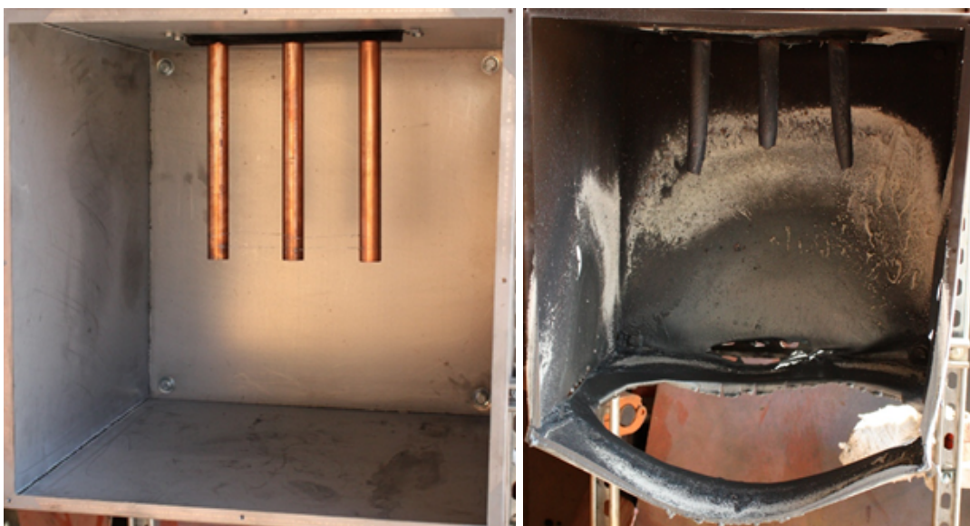
Fig. 43. Experiment OB03 pre-experiment (left) and post-experiment (right) electrodes. Phase sequence from left-to-right is C-B-A.
