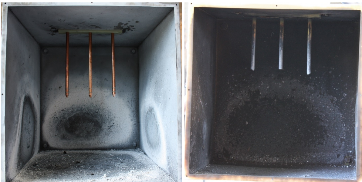
Fig. 54. Experiment OB09 pre-experiment (left) and post-experiment (right) electrodes. Phase sequence from left-to-right is C-B-A.
