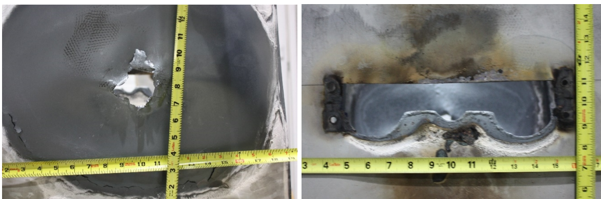
Fig. 49. Experiment OB04 enclosure breach (Left – bottom side; Right – top side)
