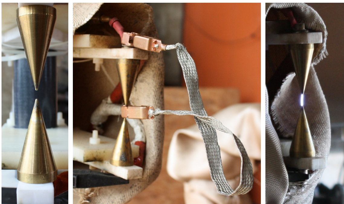
Fig. 19. Breakdown Sensor (left – electrode configuration, middle – safety jumper, right – operational experiment)
