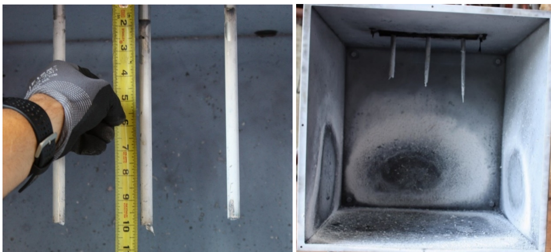
Fig. 80. Experiment OB10 Pre-experiment (left) and Post-experiment (right) electrodes. Phase sequence left-to-right (C-B-A)
