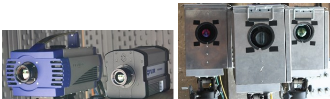
Fig. 9. Thermal imagers used inside and outside the test cell (Left – Thermal imaging cameras located approximately 30 yards from open box, Right – Imaging cameras located within the experiment cell, from left to right [thermal, high speed visible, thermal])
