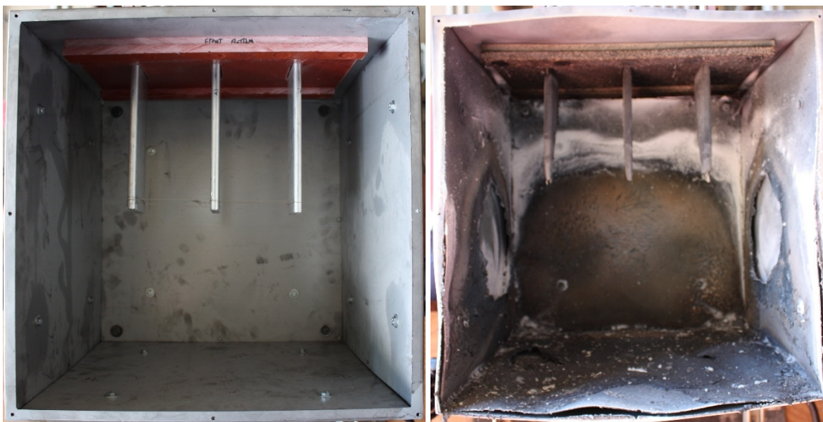
Fig. 105. Experiment OBMV02 pre-experiment (left) and post-experiment (right) aluminum electrodes. Phase sequence from left to right is C-B-A.
