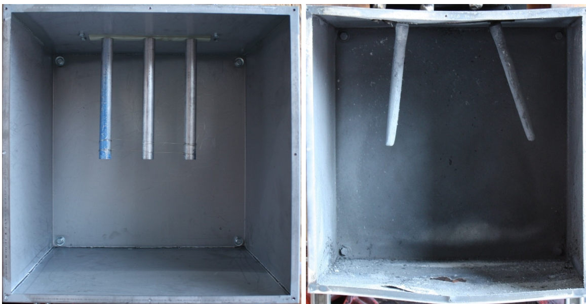
Fig. 74. Experiment OB08 pre-experiment (left) and post-experiment (right) electrodes. Phase sequence from left-to-right is C-B-A.
