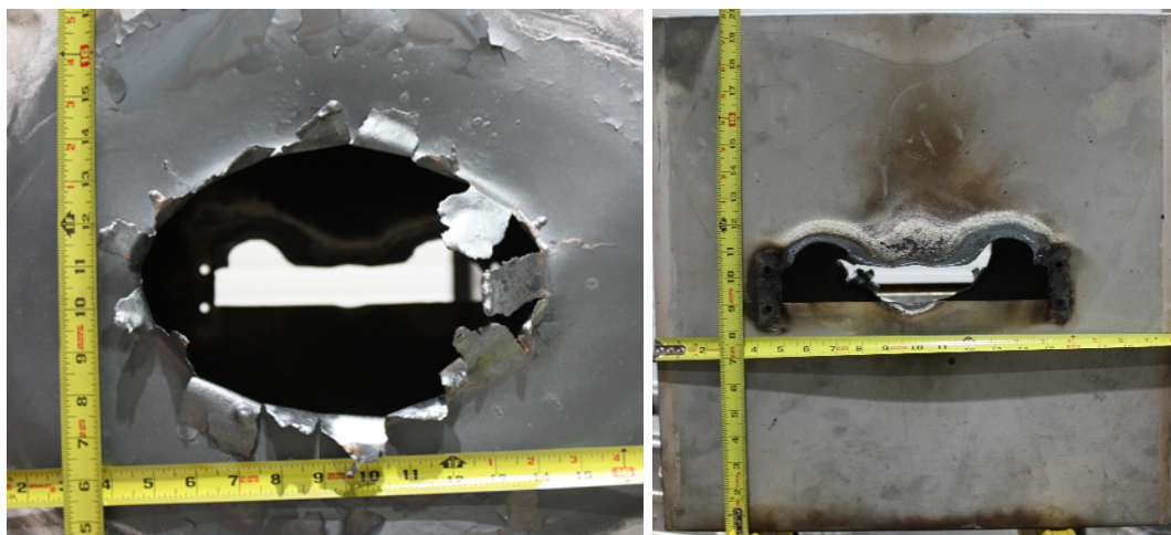
Fig. 39. Experiment OB02 enclosure breach. Bottom side breach (left), top side breach with electrode holder removed (right).
