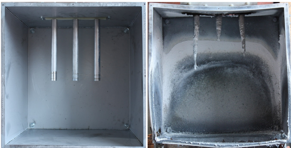
Fig. 64. Experiment OB06 pre-experiment (left) and post-experiment (right) electrodes. Phase sequence from left-to-right is C-B-A.
