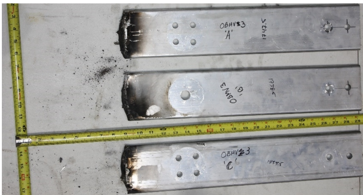
Fig. 117. Experiment OBMV03 aluminum electrode post-experiment
