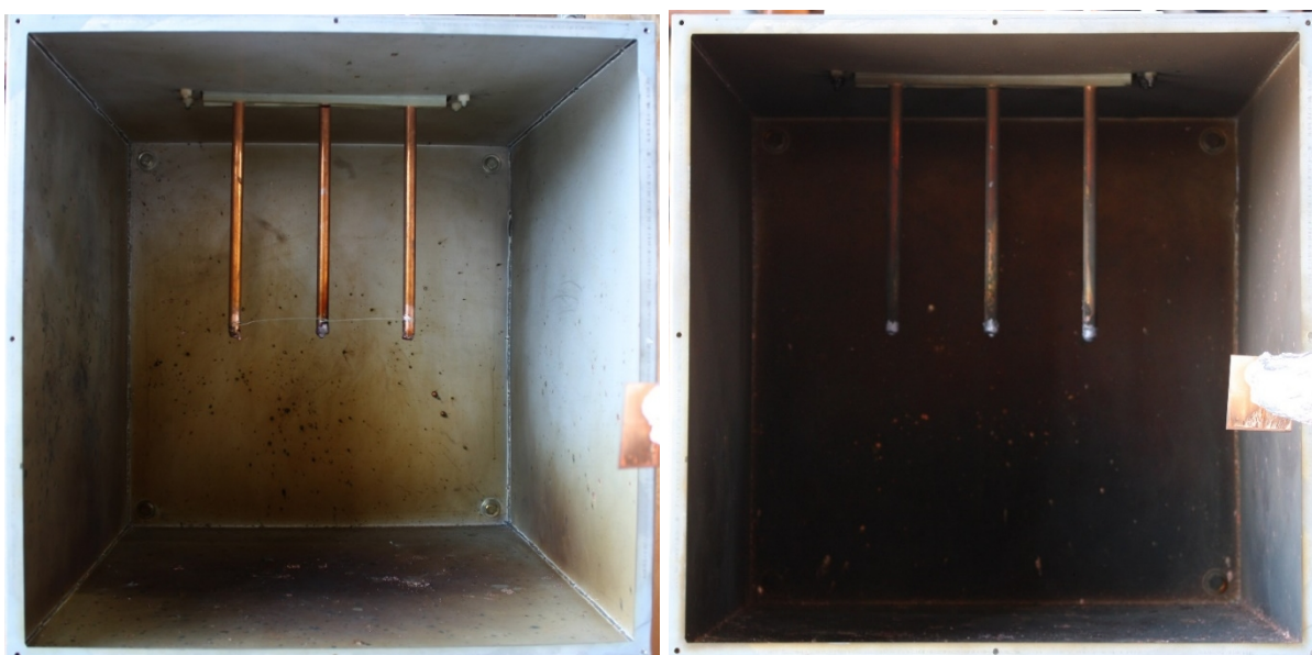
Fig. 33. Experiment OB01(b) pre-experiment (left) and post-experiment (right) electrodes. Phase sequence from left-to-right (C-B-A)
