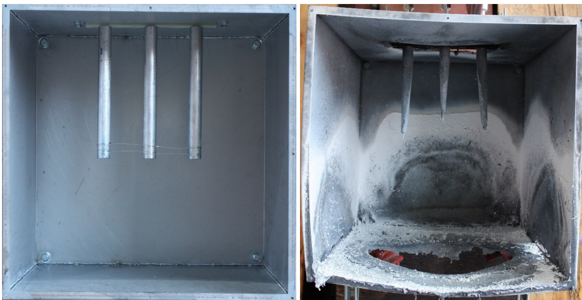
Fig. 68. Experiment OB07 pre-experiment (left) and post-experiment (right) electrodes. Phase sequence from left-to-right is C-B-A.
