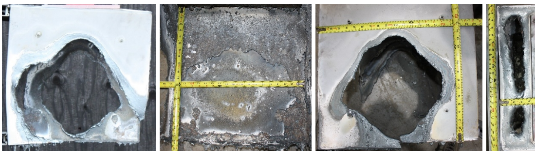
Fig. 116. Experiment OBMV03 enclosure breach (left-to-right: Left side, back side, right side, top)
