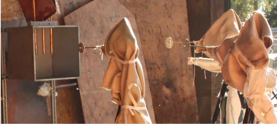
Fig. 17. d-Dot sensors arrangement prior to experiment. Note all sensors oriented in same x-direction based on results from earlier experiment indicating largest measured signal.
