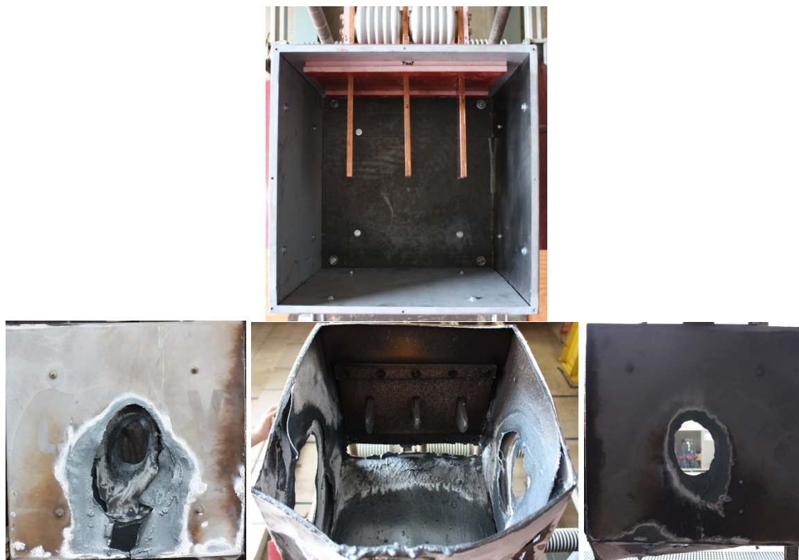
Fig. 92. Experiment OB MV05 pre-experiment (top) and post-experiment (bottom). Phase sequence from left to right is C-B-A.
