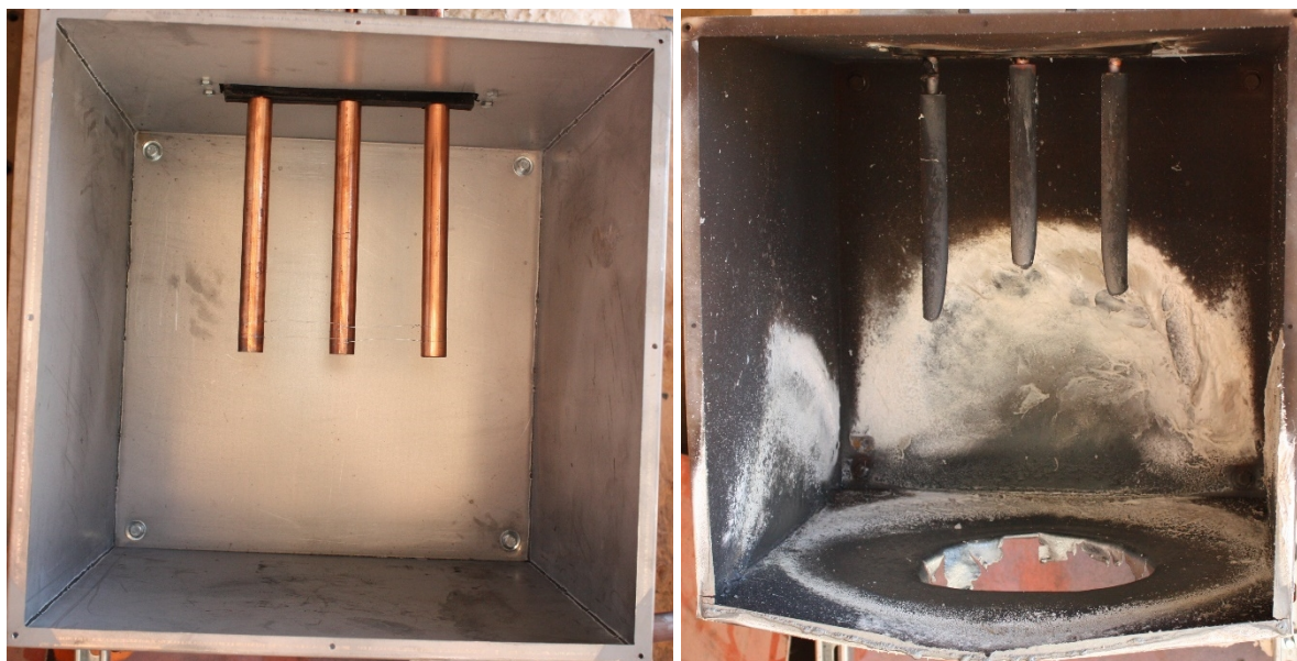
Fig. 38. Experiment OB02 pre-experiment (left) and post-experiment (right) electrodes. Phase sequence from left-to-right is C-B-A
