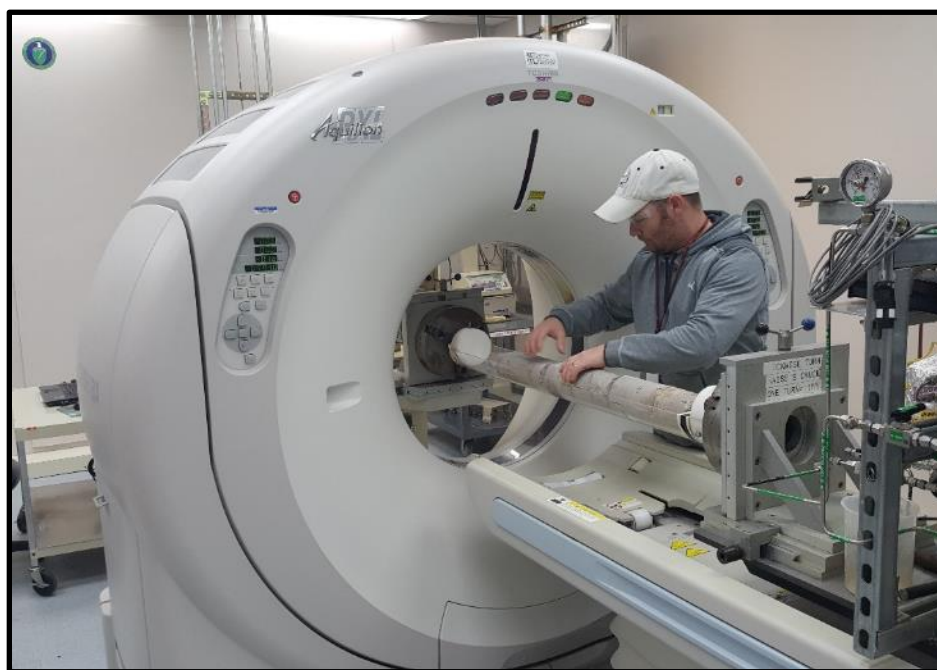
Figure 16: Toshiba Aquilion Multislice Helical CT scanner at NETL used for core analysis.
