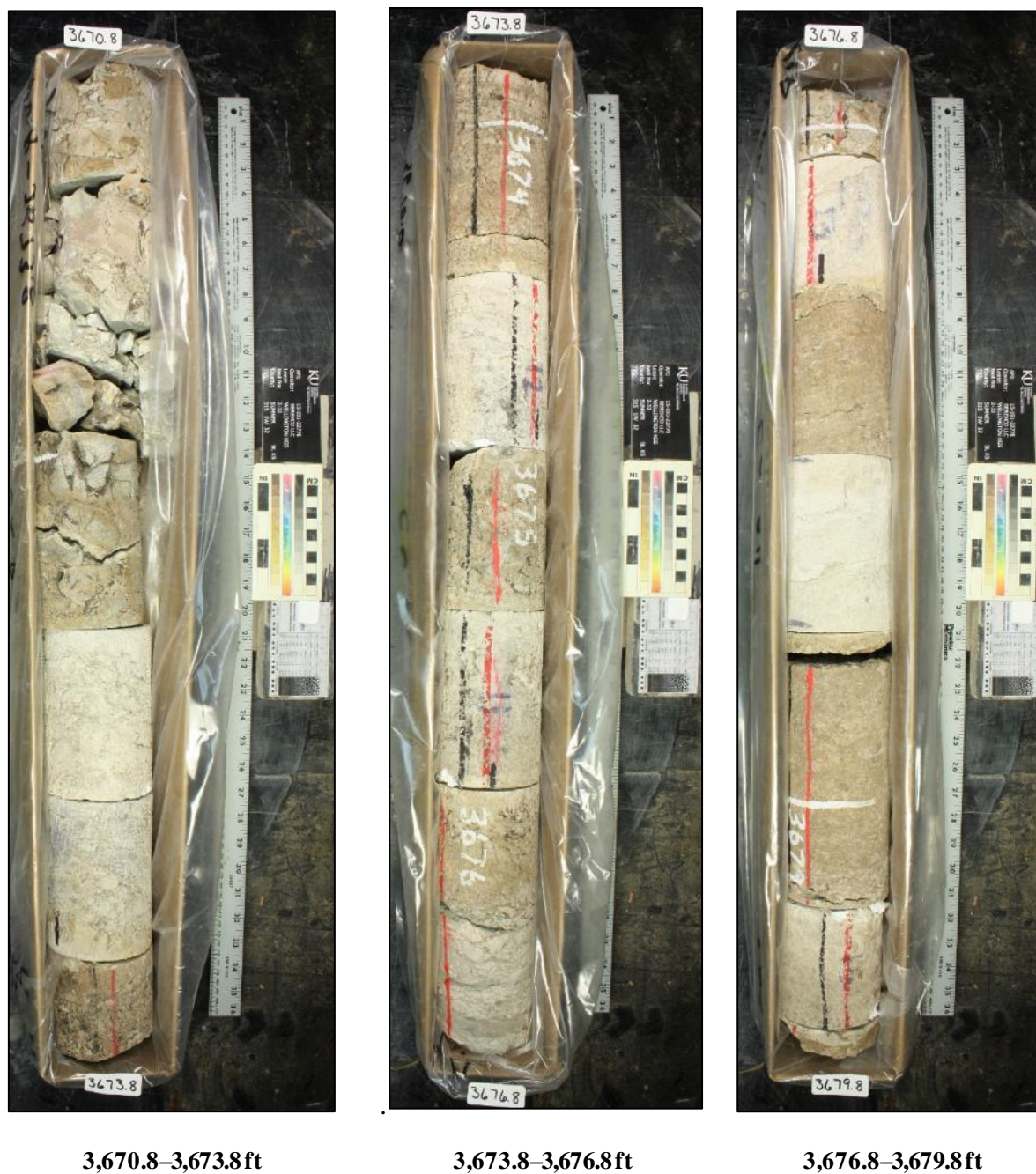
Figure 6: Wellington KGS 2-32 core photos from 3,670.8–3,679.8ft.
