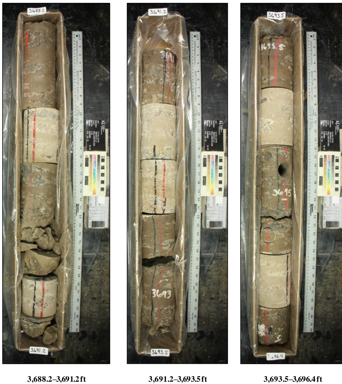
Figure 8: Wellington KGS 2-32 core photos from 3,688.2–3,696.4 ft.
