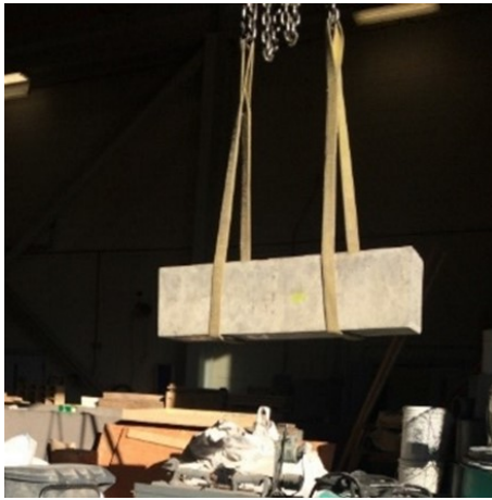
Figure 2.6: Moving specimens in the laboratory using crane and supporting carts.
