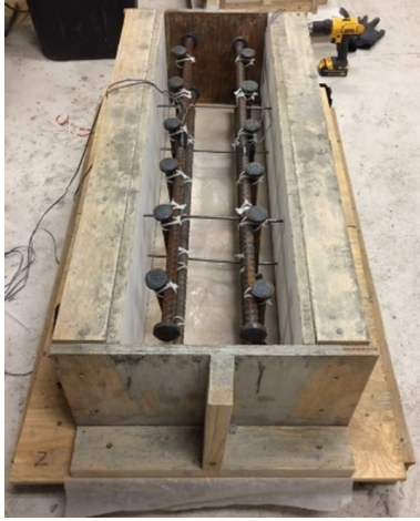
Figure 2.5: Rebar Placed in Formwork Prior to Casting
